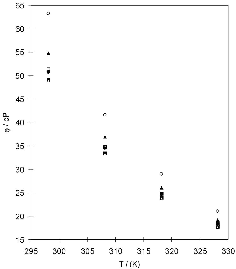
Figure 2. The viscosities of investigated oils as a function of temperature; ■, unrefined sunflower oil; Δ, refined sunflower oil; □, refined corn oil; o, olive oil; ▲, unrefined pumpkin oil; ●, salad oil.
