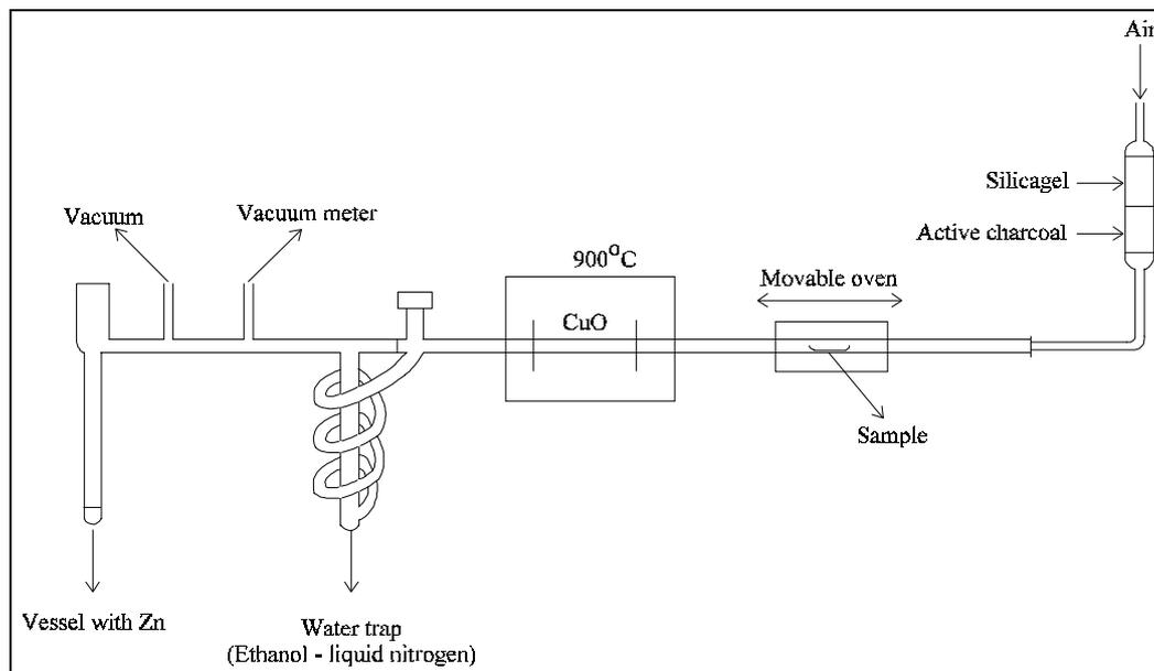
Figure 1: Schematic representation of the combustion unit
