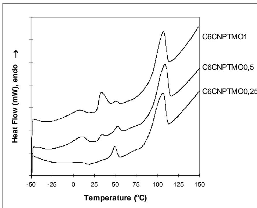
Figure 2. Normalized DSC curves (10 °C/min) of C6CNPTMOX polyurethanes with the following thermal history: heated for 5 minutes at 150 °C, then cooled to room temperature where they were held for at least one week.
