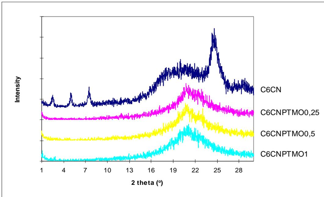
Figure 6: X-ray diffraction patterns of C6CNPTMOX polyurethanes at room temperature.
