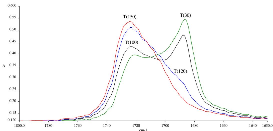
Figure 4. FTIR spectra of C6CNPTMO1 polyurethane at different temperatures T (°C) in the C=O stretching region.
