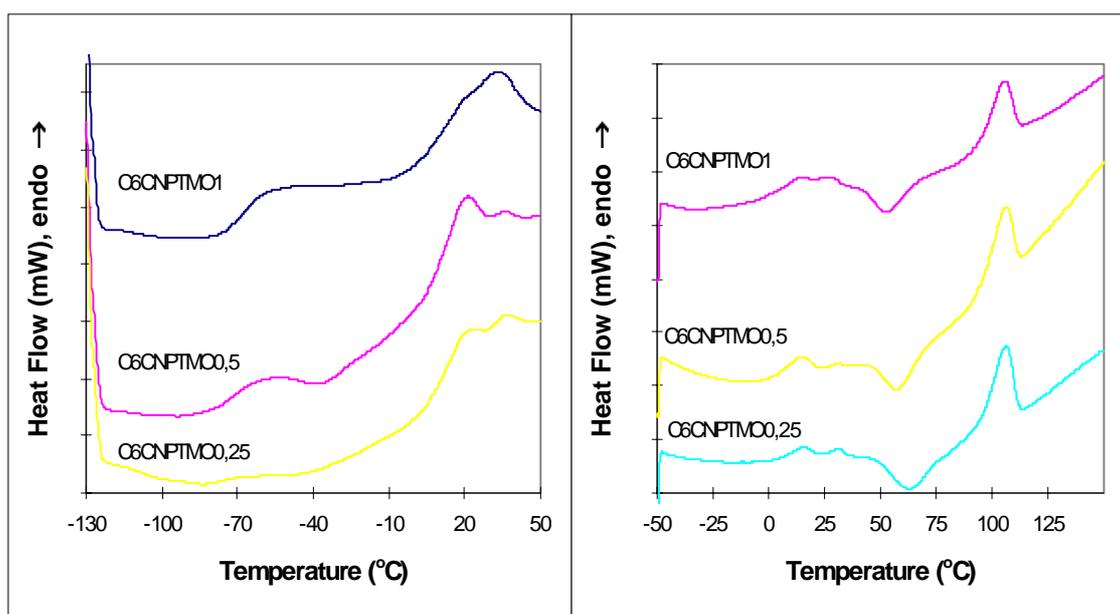
Figure 1. Normalized DSC curves of the second heating of C6CNPTMOX polyurethanes in two temperature ranges: A - heating rate of 20 °C/min, B - heating rate of 10 °C/min
