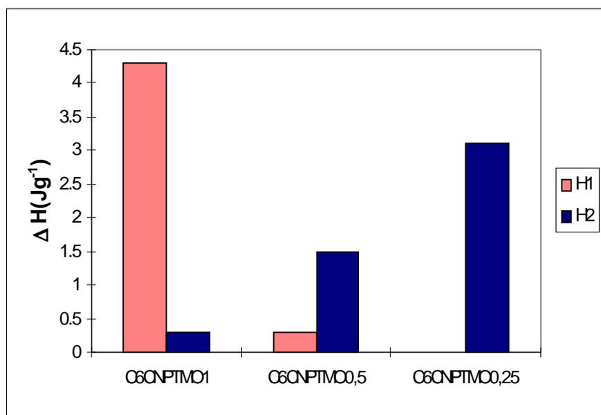
Figure 3. The dependence of  $\Delta H_1$  and  $\Delta H_2$  on the composition of C6CNPTMOX polyurethanes.
