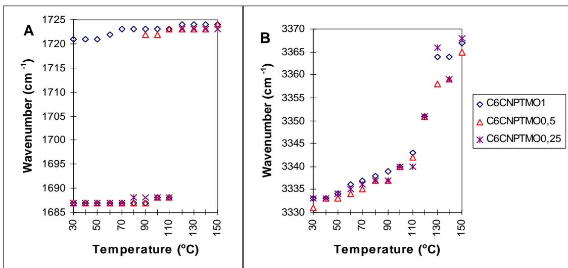
Figure 5: Shifting of the wavenumber in C6CNPTMOX polyurethanes: A - in the C=O stretching region and B - in the N-H stretching region.
