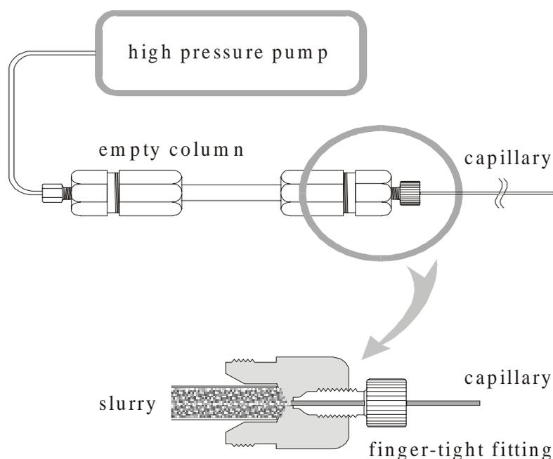
Figure 1: Schematic representation of the packing assembly and a detailed arrangement of capillary and the slurry reservoir.
