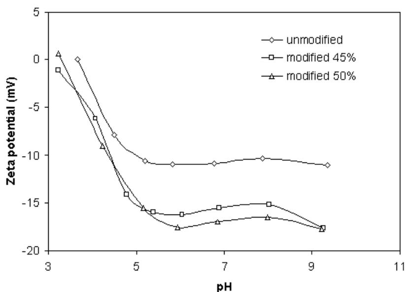
**Scheme 4.** Dependencies of the zeta potential on pH for sulfonized polysulfone membranes.
