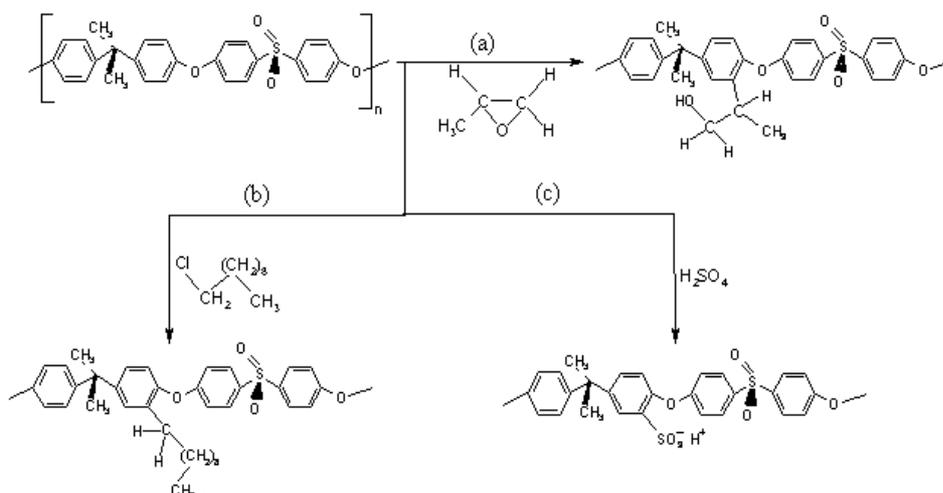
**Scheme 1.** Chemical modifications of the surface of polysulfone membranes. The Friedel-Crafts electrophilic substitution of aromatic rings in polysulfone molecule (a) with propylene oxide and (b) with 1-chlorodecane, (c) sulfonation with sulfuric (VI) acid water solution.
