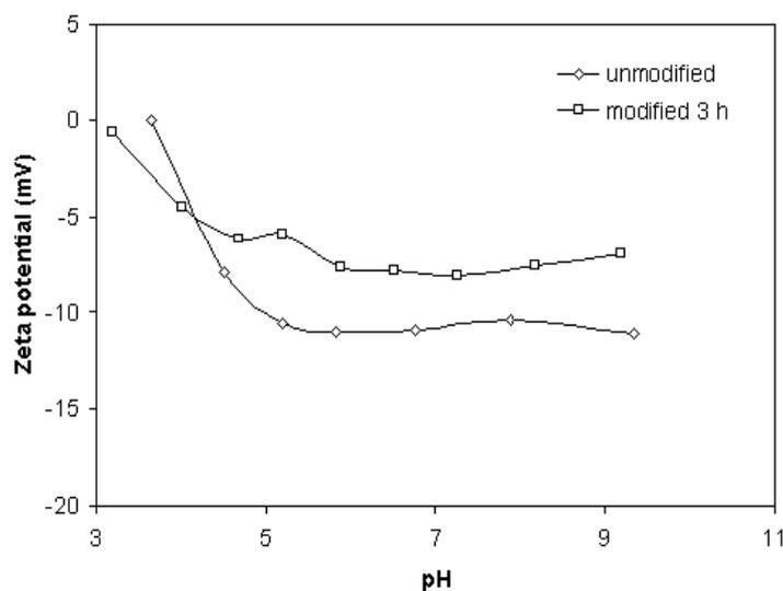
**Scheme 3.** Dependencies of the zeta potential on pH for polysulfone membranes modified by Friedel-Crafts reaction with 1-chlorodecane.
