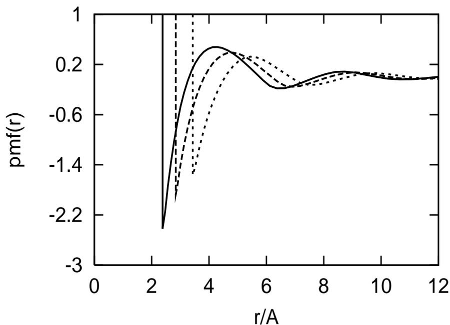
Figure 1: Ion-water (oxygen site) potential of mean force for  $Li^+$  ion (full line), cation of the reference electrolyte (dashed line), and  $Cs^+$  ion (dotted line) as calculated by the CSL integral equation theory.
