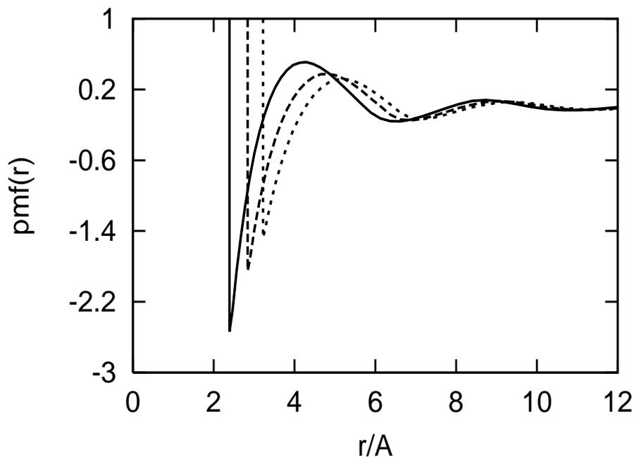
Figure 2: Ion-water (hydrogen site) potential of mean force for  $F^-$  ion (full line), anion of the reference fluid (dashed line), and  $I^-$  ion (dotted line), as calculated by the CSL integral equation theory.
