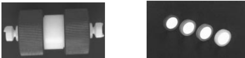
Figure 1: CIM ® disk housing and CIM ® disks. CIM ® disk (right) consist of the white monolith in the middle of the disk and of a non-porous self-sealing ring. Different colors represent different chemistries. CIM ® disk is placed in a CIM ® housing (left) and used as a chromatographic column.
