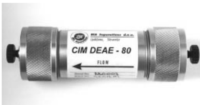
Figure 8. CIM 80 ml monolithic column. Tube shaped monolith in placed in a stainless still housing. Flow rates up to 250 ml/min can be used.
