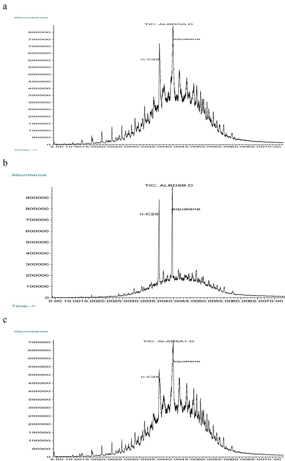
**Figure 1.** The total ion chromatogram (a) of motor oil (concentration  $83 \text{ mg mL}^{-1}$ ) and of biotic (b) and abiotic (c) samples after 5 days of incubation.
