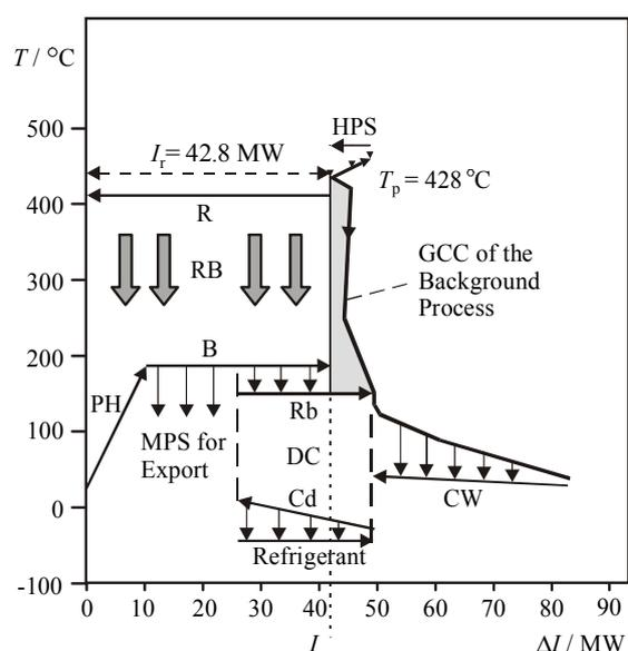
Figure 3: Extended grand composite curve of base process flowsheet
