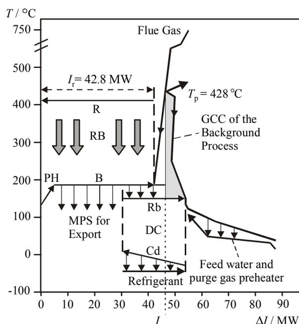
Figure 5: Extended grand composite curve of modified process flowsheet
