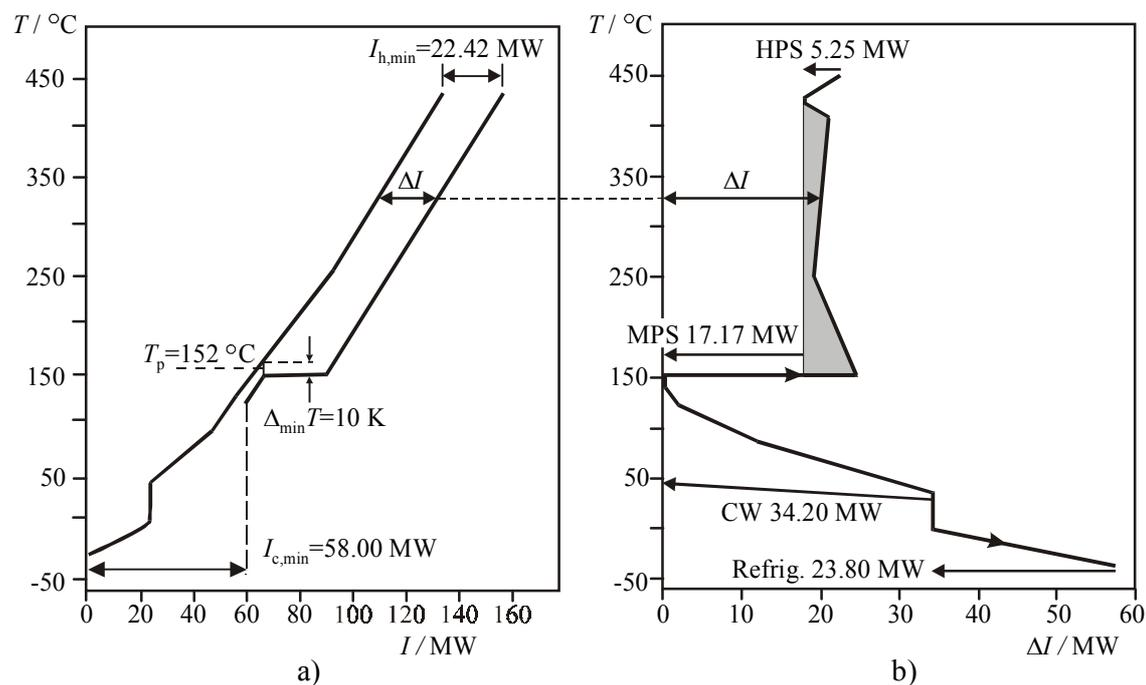
Figure 2: Composite curves a) and grand composite curve b) of HEN in the base flowsheet of ammonia process
