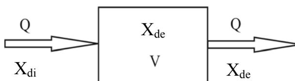
**Figure 3 – Flow chart for a completely mixed aerobic digester**
