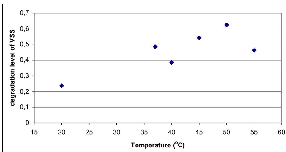
**Figure 6 – Temperature dependence of aerobic degradation (cross-section of Figure 5 at 17 days as a function of temperature)**
