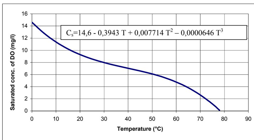
**Figure 2 – Oxygen solubility in water at normal pressure**
