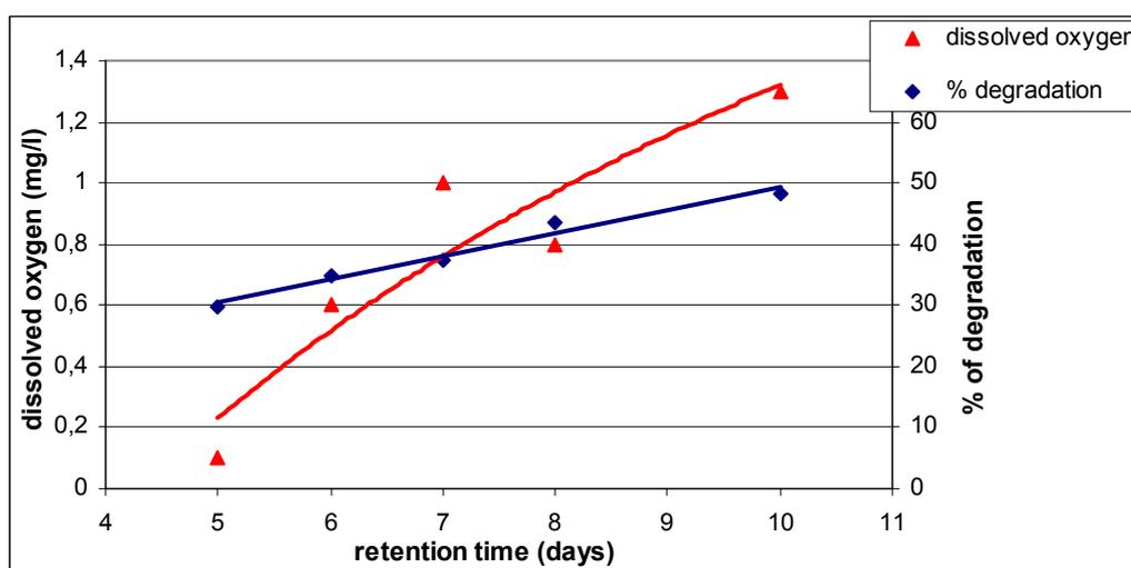
**Figure 10 – dissolved oxygen and % of degradation in aerobic digestion as a function of HRT**
