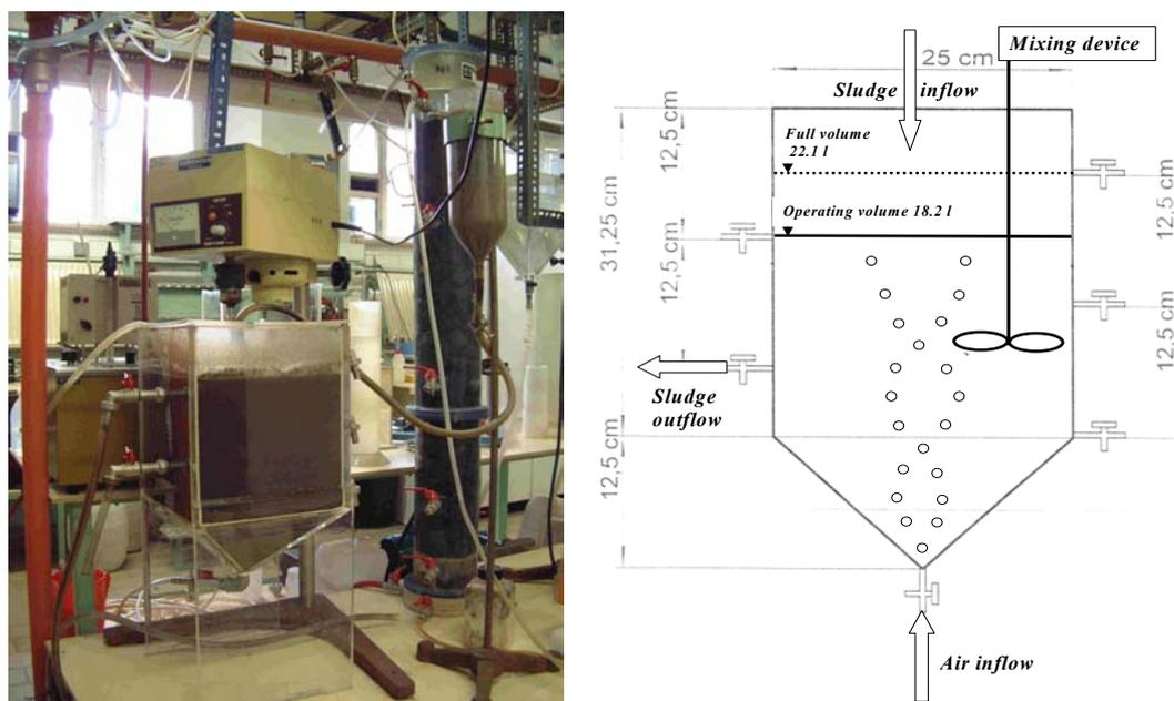
**Figure 4 – Aerobic reactor used for experiments.**
