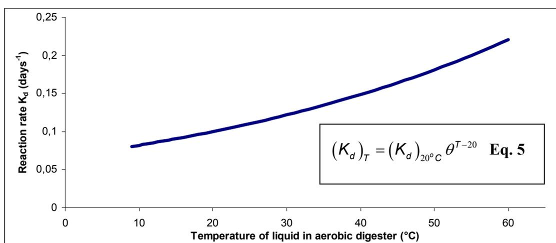
**Figure 1 – Aerobic digestion reaction rate as a function of temperature**
