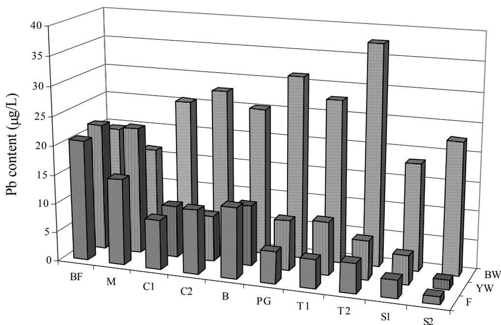
**Figure 5.** Pb content in some stages of winemaking process. Sample labels: F; for white grape varieties must after clarification and for red grape varieties the liquid fraction taken at the sixth day of maceration, YW: young wine, BW: bottled wine, BF: Blaufränkisch, M: Merlot, C1, C2: Cabernet Sauvignon, B: Barbera, PG: Pinot gris, T1,T2: Gewürztraminer, S1, S2: Sauvignon.
