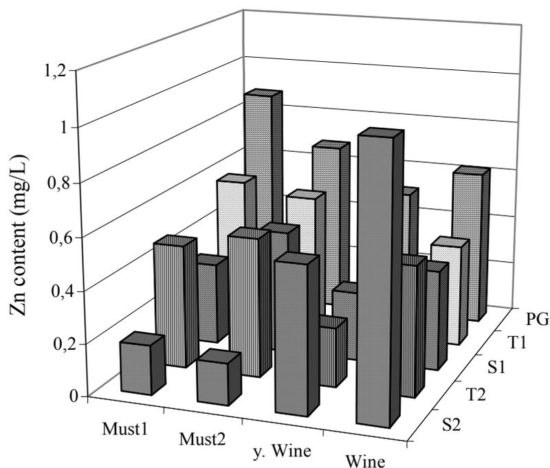
**Figure 3.** The Zn migration during white wine production. Sample labels: Must1: must before clarification, Must2: must after clarification, y. Wine: young wine, Wine: bottled wine, S1, S2: Sauvignon, PG: Pinot gris, T1,T2: Gewürztraminer.
