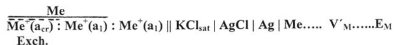
Figure 4. Galvanic cell representations corresponding to the proposed method; three cells with two solutions and three with a suspension. The line, double line and dashed line have their common meaning; a single line with parallel dashed line means the electrode in intense contact with particles causing double layer overlapping. The position of the last symbol shows the cell phase in contact with the electrode. Symbol a_{\text{dl}} means ion activity in particle double layer and a_{\text{cr}} the activity in the contact region.
