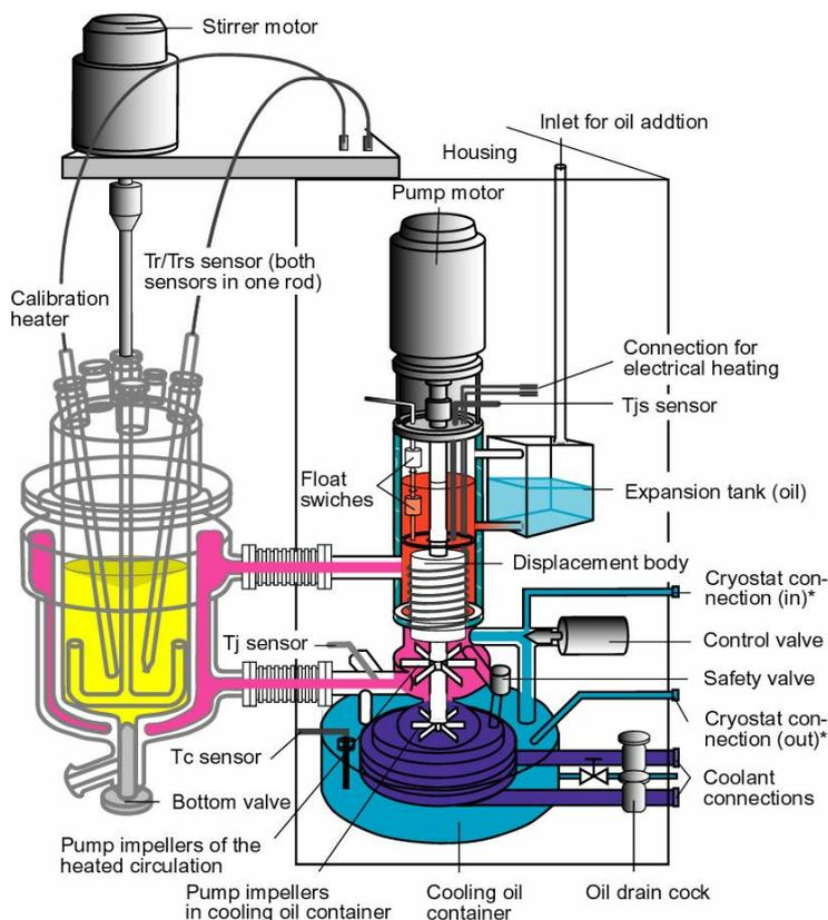
**Figure 1.** Reaction calorimeter with heat flow balancing.
