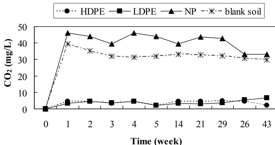
**Figure 4.** Carbon dioxide production during the biodegradation of high density polyethylene (HDPE), low density polyethylene (LDPE) and degradable polyethylene (NP) films and in blank soil.
