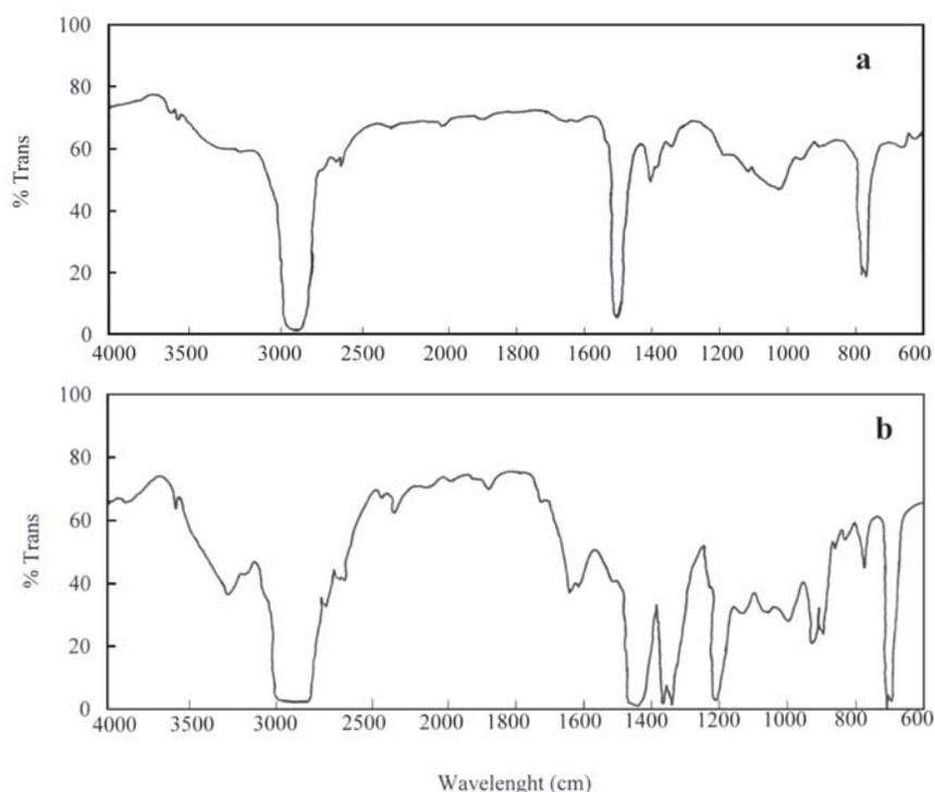
**Figure 5.** Infrared spectrum of degradable polyethylene (NP) films before soil burial (a) and after 60 weeks of soil burial (b).
