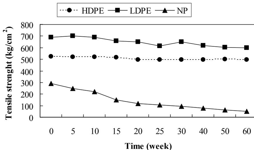
**Figure 3.** Tensile strength of high density polyethylene (HDPE), low density polyethylene (LDPE) and degradable polyethylene (NP) films during soil burial.
