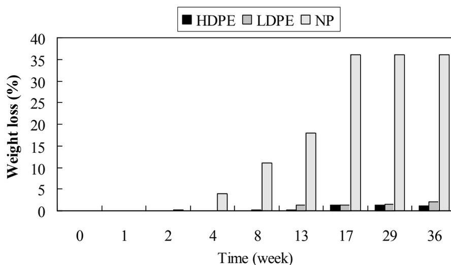
**Figure 1.** Weight loss (%) of high density polyethylene (HDPE), low density polyethylene (LDPE) and degradable polyethylene (NP) films during soil burial.
