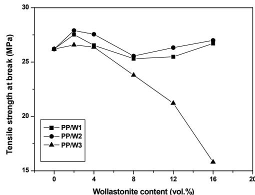
Figure 4. Tensile strength at break of the PP/wollastonite composites in dependence of wollastonite content.
