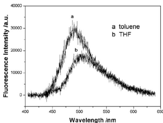
Figure 4. TPEF spectra of BCST in THF and toluene.
