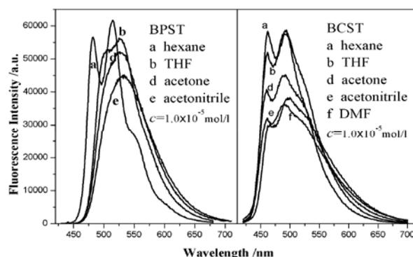
**Figure 2.** Fluorescence spectra of BPST and BCST in different solvent.
