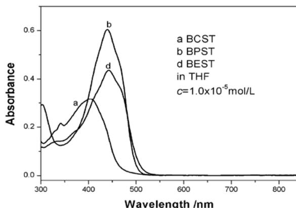
**Figure 1.** Absorption spectra of BEST, BPST and BCST in THF.
