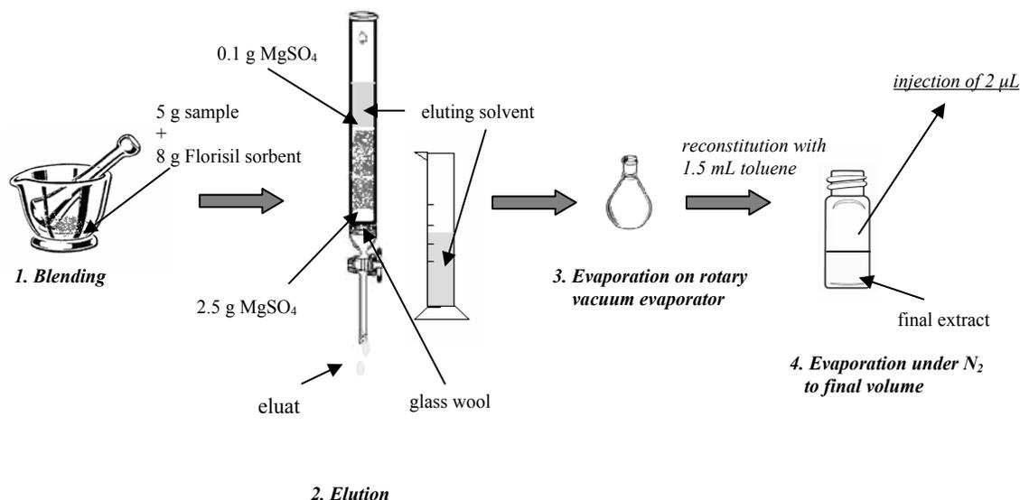
Figure 1. Scheme of the whole apple sample MSPD preparation process.
