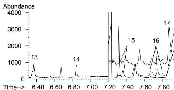
**Figure 5.** Extracted chromatograms of target ions of pesticides in matrix matched standard solution from fast GC-MS measurements; concentration of pesticides 10  $\mu\text{g kg}^{-1}$ . 1: dimethoate, 2: terbutylazine, 3: diazinon, 4: pyrimethanil, 5: chlorpyrifos-methyl, 6: fenitrothion, 7: chlorpyrifos, 8: cyprodinyl, 9: penconazole, 10: methidathion, 11: kresoxim-methyl, 12: myclobutanil, 13: tebuconazole, 14: phosalone, 15: bitertanol, 16: cypermethrin, and 17: etofenprox.
