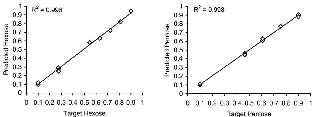
**Figure 4.** Comparison of predicted results from the NN5 model with target values from the actual values hexose and pentose for the testing data set.
