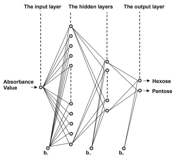
Figure 1. Network architecture used in the spectrophotometric method.
