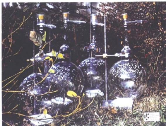
Figure 1. Photochemical synthesis of XeF<sub>2</sub>
