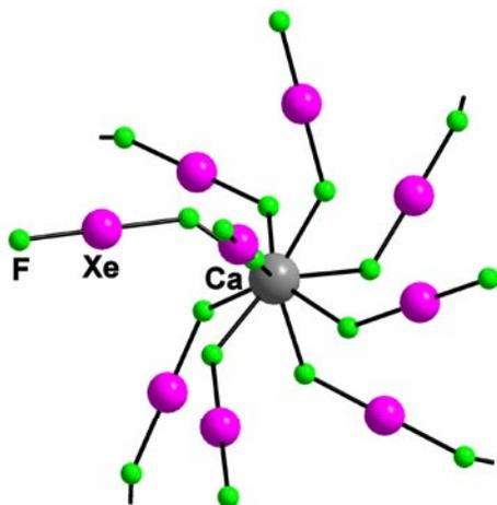
**Figure 11.** Example of the metal coordinated only by  $\text{XeF}_2$  (bridging and non-bridging); one  $\text{Ca}^{2+}$  centre in  $[\text{Ca}_2(\text{XeF}_2)_9](\text{AsF}_6^-)_4$ .<sup>74</sup>
