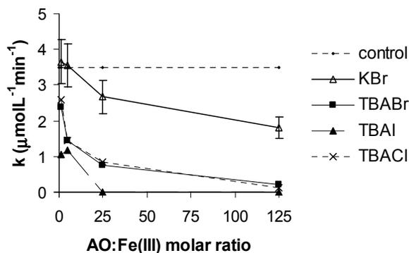
**Figure 6.** Effect of concentration of halide (AO) in Fenton-like reaction mixture containing Fe(III) ions as catalyst on the rate of NPG hydroxylation. The control sample contained no antioxidant, other samples contained potassium bromide (KBr), tetrabutylammonium bromide (TBABr), tetrabutylammonium iodide (TBAI) and tetrabutylammonium chloride (TBACl). Error bars represent standard deviation for determination of rate constants.
