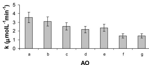
**Figure 7.** Effect of various bromides (AO) with bromide:Fe(III) molar ratio 5:1 on the rate of hydroxyl radical production in the pseudo-Fenton reaction mixture containing NPG. Sample a contained potassium bromide, b-methyltriphenyl phosphonium bromide, c-benzyltributylammonium bromide, d-tetraethylammonium bromide, e-tetrapropylammonium bromide, f-tetrabutylammonium bromide and g-dodecyltrimethylammonium bromide. Error bars represent standard deviation for determination of rate constants.
