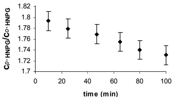
**Figure 3.** *p*-HNPG/*o*-HNPG product ratio for pseudo-Fenton reaction system containing iron(III) during 100 min of reaction at 70 °C.
