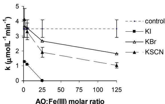
**Figure 5.** The effect of concentration of halides and a pseudo-halide in Fenton-like reaction mixtures containing Fe(III) ions as catalysts on the rate of NPG hydroxylation. The control sample contained no antioxidant (AO), KI represents addition of potassium iodide, KBr addition of potassium bromide and KSCN addition of potassium thiocyanate. Error bars represent standard deviation for determination of rate constants.
