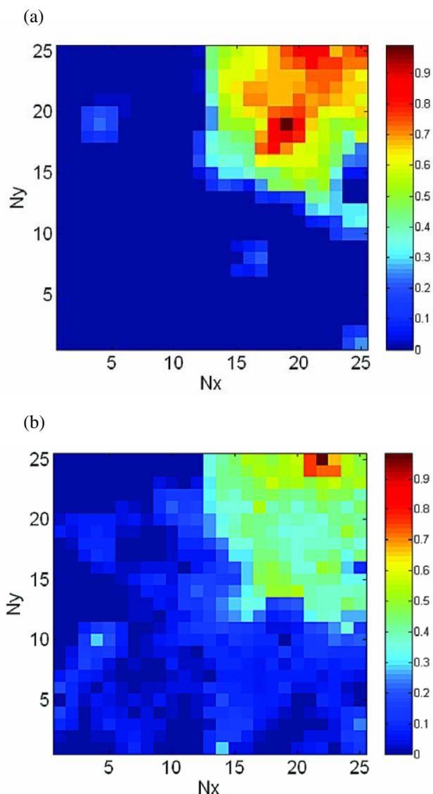
Figure 7. The weights in the 6<sup>th</sup> Kohonen level corresponding to Cr(VI) (a) and in the 7<sup>th</sup> Kohonen level corresponding to Cr total (b).
