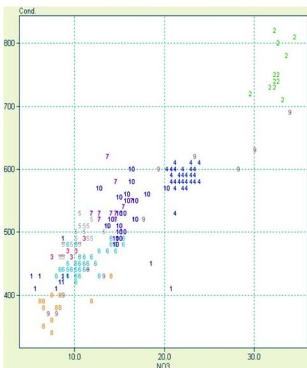
**Figure 1.** Correlation between nitrate content ( $\text{NO}_3^-$ ) and electrical conductivity. The sampling sites (classes) are denoted by numbers from 1 to 10.
