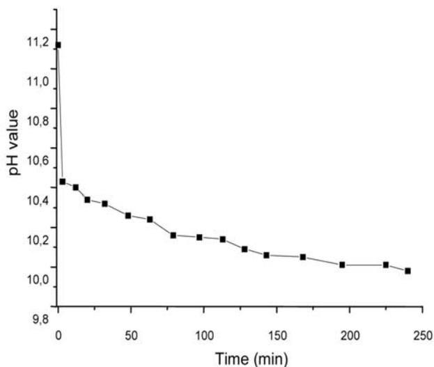
**Figure 2.** Changes of pH of ethanolamine ( $w_{EA} = 0.721\%$ ) spruce sawdust mixture during 4 h of soaking.
