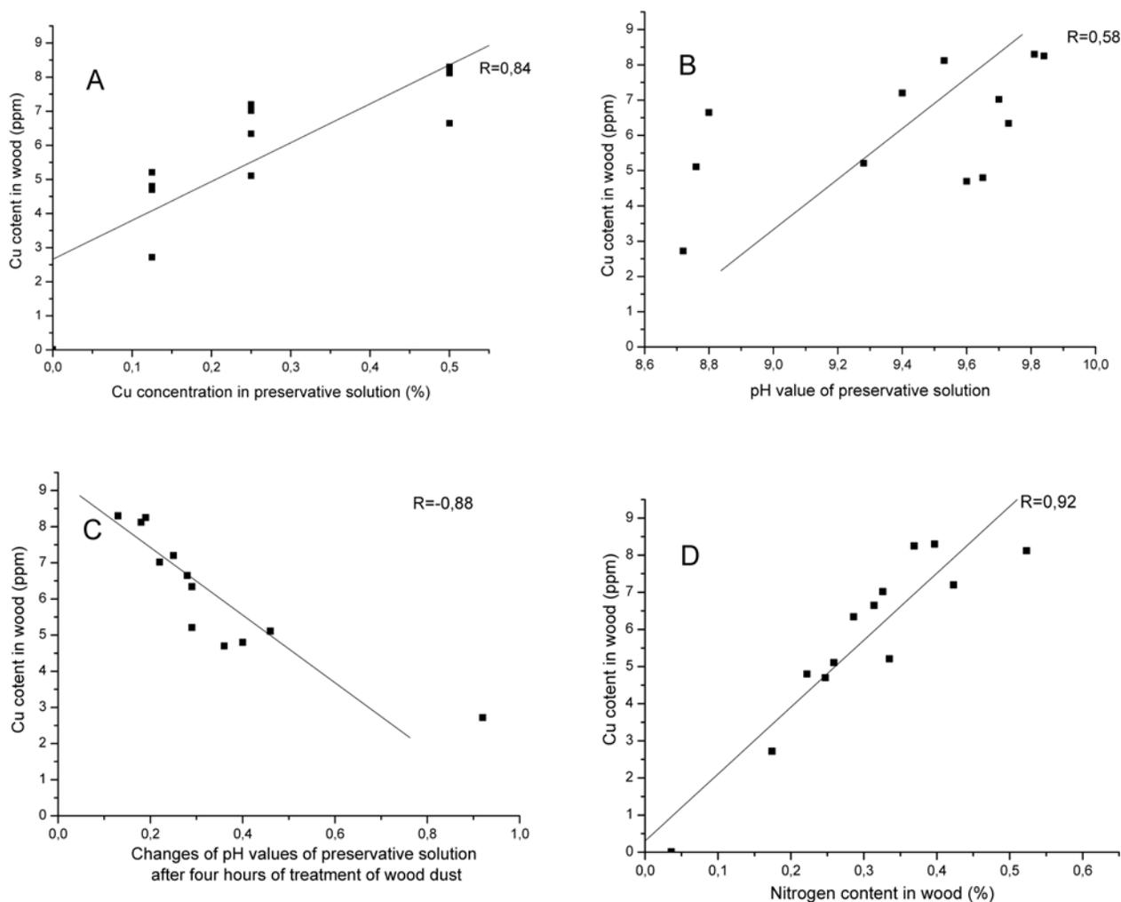
**Figure 1.** Correlations between copper content in immersed wood and preservative solution concentration (A), pH of preservative solution (B), changes of pH after 4 h of immersion (C) and nitrogen content in immersed wood (D).
