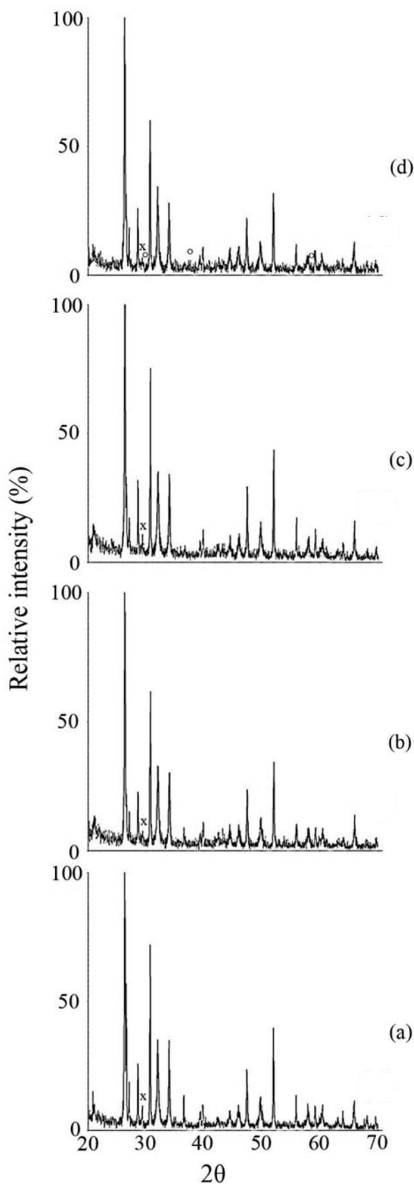
**Figure 6.** XRD patterns of different samples: sample 2 (a), sample 3 (b), sample 4 (c) and sample 5 (d). The secondary phases are marked:  $\text{CaCO}_3$  (x) and  $\text{MnO}_2$  ( $\square$ ).
