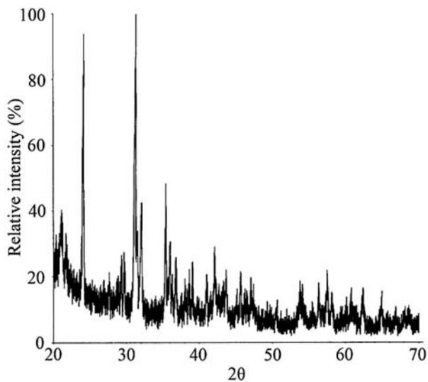
Figure 9. XRD pattern of malachite.
