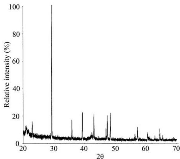
**Figure 2.** XRD pattern of CaCO<sub>3</sub>.
