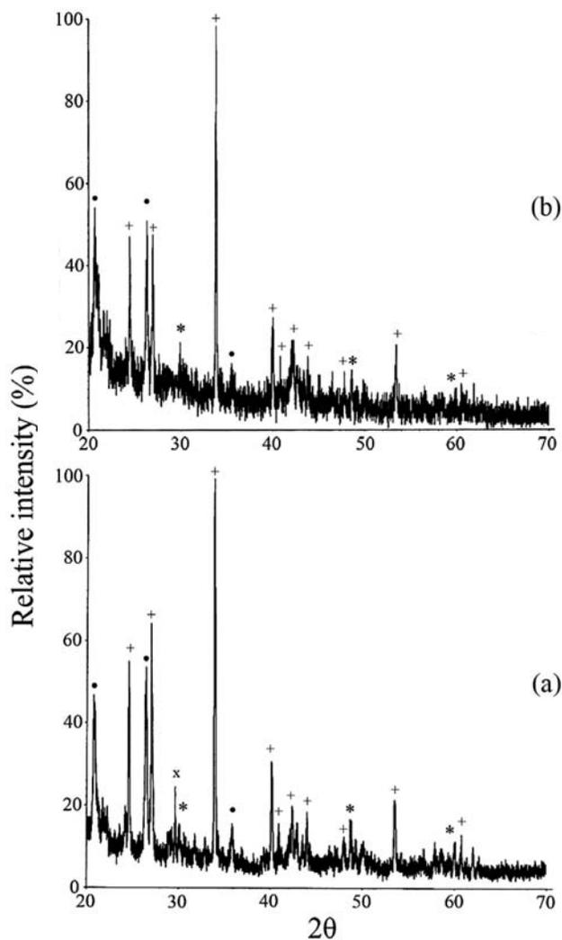
Figure 10. XRD patterns of sample 8 (a) and sample 9 (b). The main and secondary phases are marked:  $\text{PbCO}_3 \times \text{Pb(OH)}_2$  (+),  $\text{SiO}_2$  (•),  $\text{Sb}_2\text{O}_3 \times 2\text{PbO}$  (\*), and  $\text{CaCO}_3$  (x).
