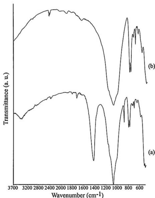
**Figure 16.** FTIR spectra of sample 8: just obtained (a) and fired at 1000 °C (b).
