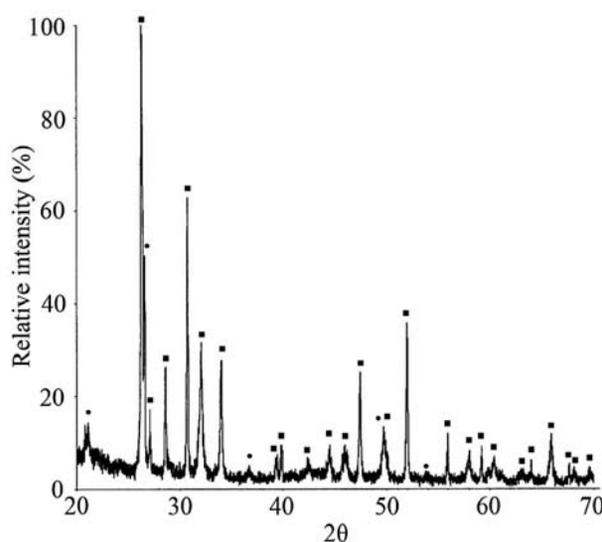
**Figure 1.** XRD pattern of the mixture of Pb<sub>3</sub>O<sub>4</sub> (■) : SiO<sub>2</sub> (●) = 3.625 : 0.875.
