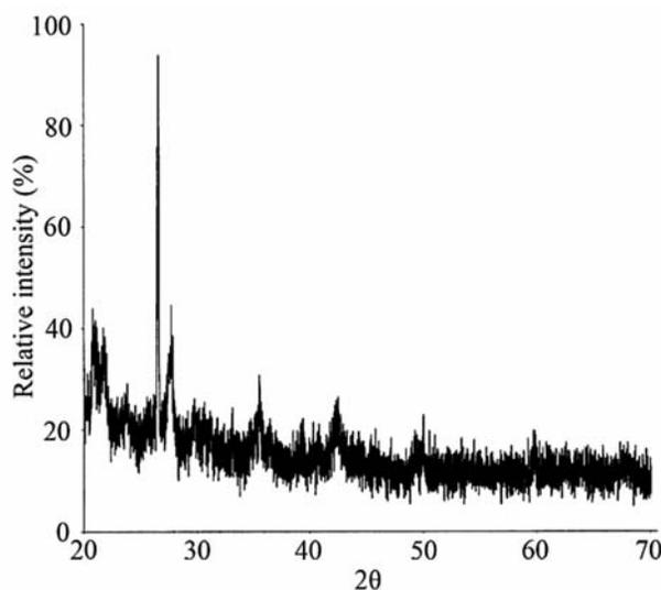
Figure 13. XRD pattern of pottery calcined at  $1000^\circ\text{C}$ .
