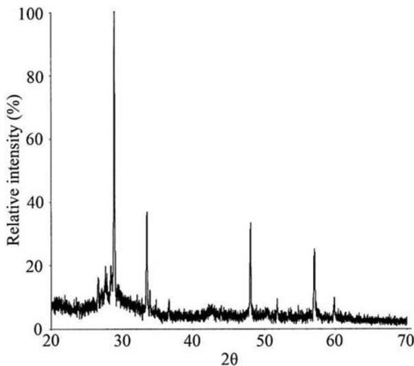
Figure 3. XRD pattern of lead-tin yellow.
