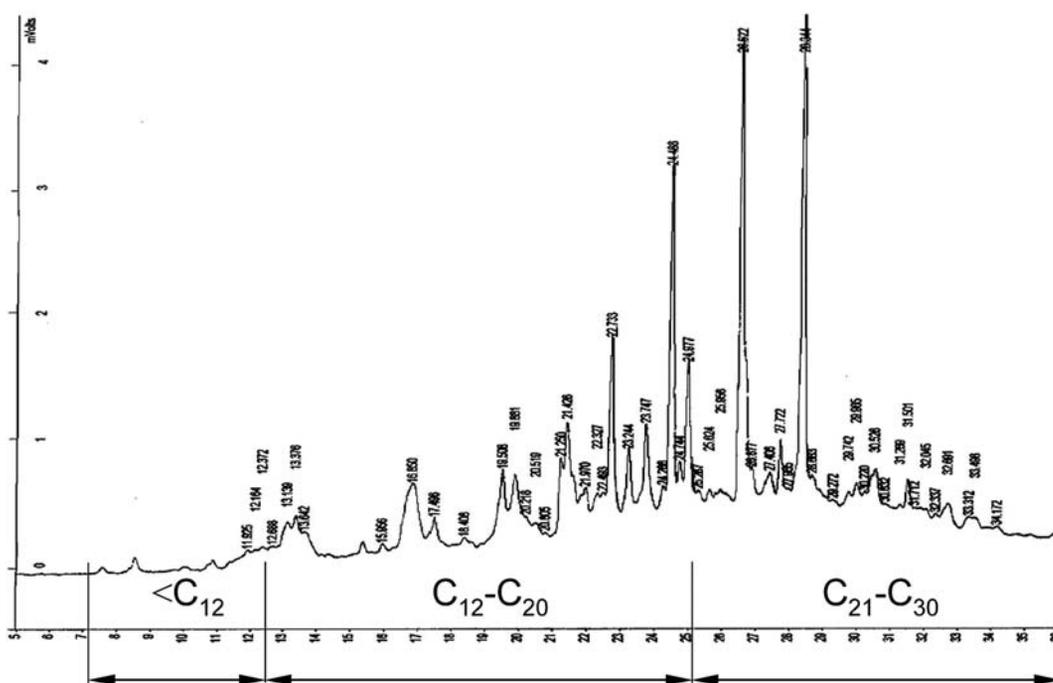
**Figure 1.** Chromatogram of the aliphatic hydrocarbon (AH) fraction contained in a complex hydrocarbon mixture extracted from the PR soil containing 60,600 mg kg<sup>-1</sup> TPH. GC was implemented with an FID and a non-polar 007 fused silica capillary column: 25 m, i.d. 0.53 mm and film thickness 1  $\mu$ m.
