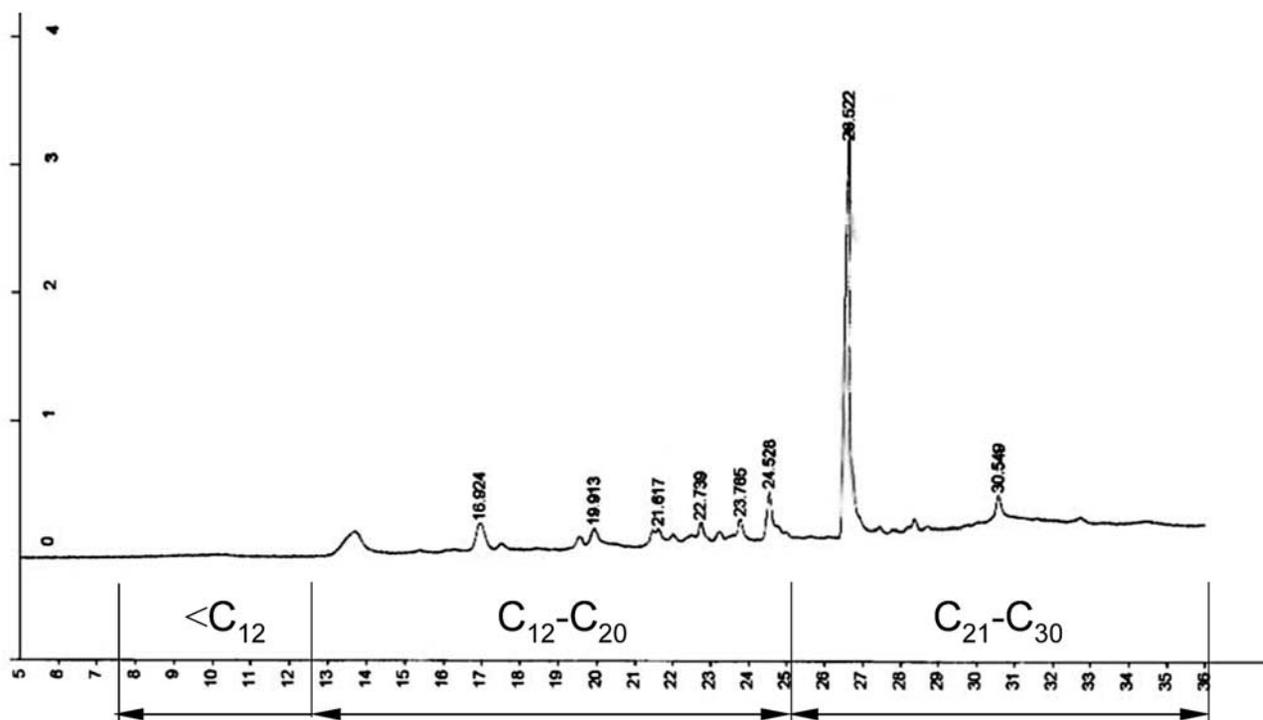
**Figure 3.** Chromatogram of the residual aliphatic hydrocarbon (AH) fraction analysed after biotreatment with *A. sydowii*. GC implemented with an FID and a non-polar 007 fused silica capillary column: 25 m, i.d. 0.53 mm and film thickness 1 µm.
