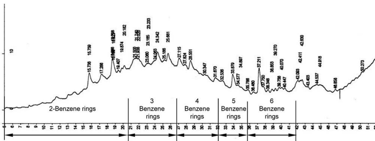
**Figure 4.** Chromatogram of residual polycyclic aromatic hydrocarbons (PAHs) fraction after biotreatment with *A. Sydowii*. GC implemented with an FID and a non-polar 007 fused silica capillary column: 25 m, i.d. 0.53 mm and film thickness 1  $\mu$ m.
