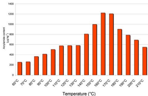
Figure 2. Dependence of acrylamide formation on kilning temperature.
