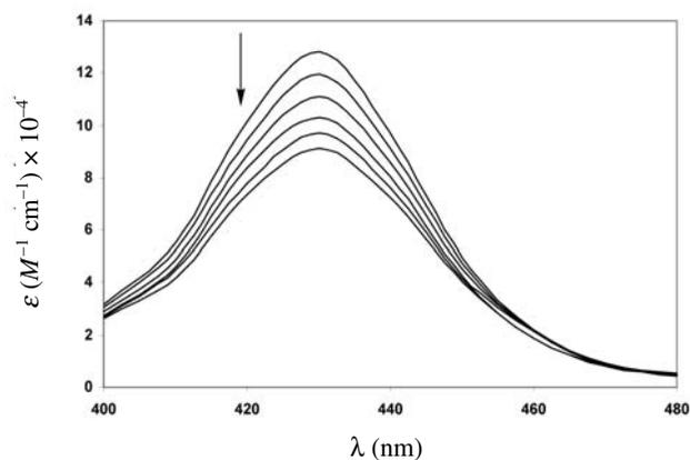
**Fig. 1:** The spectrophotometric titration of CuTBzPyP with DNA in 5 mM phosphate buffer, pH 7.0 and at 25 °C. The concentration of DNA increases in the direction of arrow and the concentration of porphyrin in the cell was  $3.68 \times 10^{-6}$  M.
