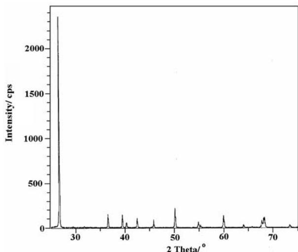
Figure 2. XRD spectrum of untreated tripoli.
