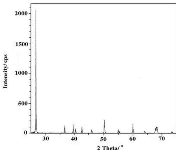
Figure 1. XRD spectrum of untreated tripoli.
