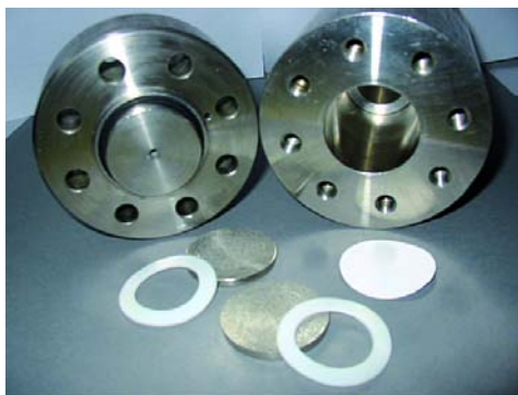
Figure 5: High pressure continuous enzymatic flat-shape membrane reactor with sintered plates and flat membrane.
