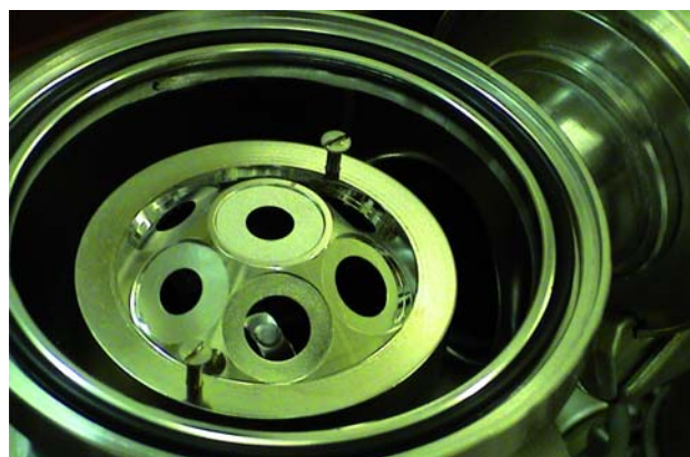
Fig. 9: Compact vacuum evaporation/sublimation cell with mask for seven source substrates and tungsten filament.
