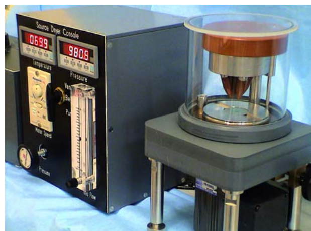
Fig. 4: IRMM's drying device for drop-deposited radioactive sources, with control unit. The source is placed on a turntable and dried by the injection of heated nitrogen through four jets, inside a bell jar connected to a vacuum pump.
