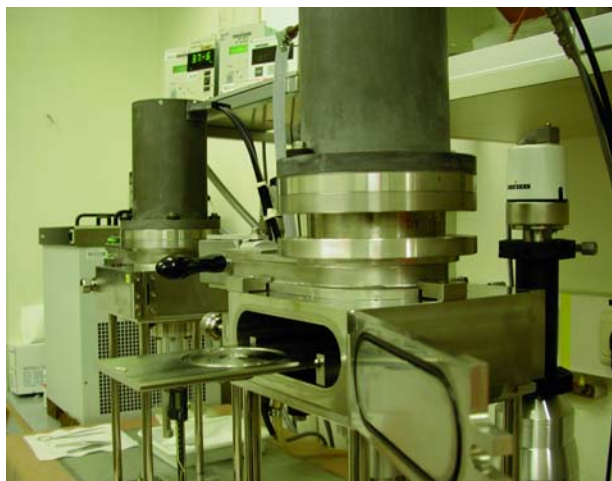
Fig. 5: Picture of set-up for high-resolution alpha-particle spectrometry.
