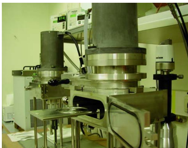
Fig. 5: Picture of set-up for high-resolution alpha-particle spectrometry.
