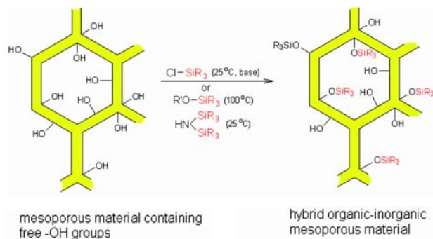
Figure 1. Mesoporous silicates functionalization by post-synthesis method.
