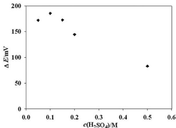
**Figure 4.** Effect of  $\text{H}_2\text{SO}_4$  concentration on the change of potentials. Experimental condition:  $c(\text{NAC}) = 5.0 \times 10^{-5}$  M,  $c(\text{KI}) = 5.0 \times 10^{-6}$  M,  $c(\text{KIO}_3) = 1.0 \times 10^{-4}$  M. Final volume: 25.0 mL
