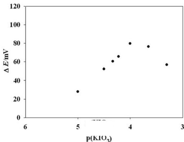
**Figure 3.** Effect of  $\text{KIO}_3$  concentration on the change of potentials. Experimental condition:  $c(\text{NAC}) = 5.0 \times 10^{-5}$  M,  $c(\text{KI}) = 5.0 \times 10^{-5}$  M,  $c(\text{H}_2\text{SO}_4) = 0.1$  M. Final volume: 25.0 mL
