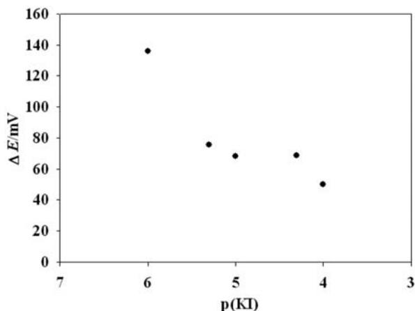
**Figure 2.** Effect of KI concentration on the change of potentials. Experimental condition:  $c(\text{NAC}) = 5.0 \times 10^{-6}$  M,  $c(\text{KIO}_3) = 1.0 \times 10^{-4}$  M,  $c(\text{H}_2\text{SO}_4) = 0.1$  M. Final volume: 25.0 mL
