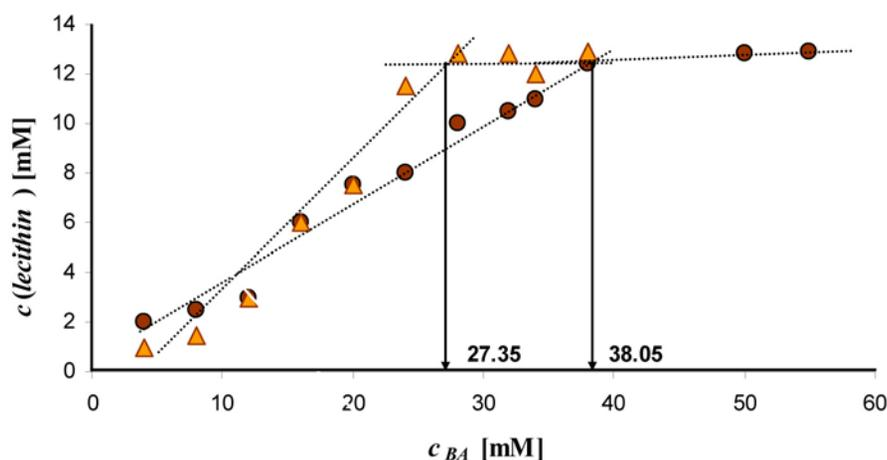
**Figure 6.** Solubilization of lecithin with Na-12-MKC. I: D<sub>2</sub>O solution, II: D<sub>2</sub>O solution saturated with 1-octanol.
