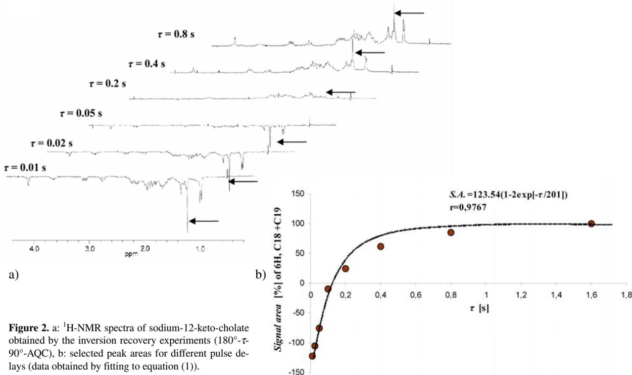
**Figure 2.** a:  $^1\text{H}$ -NMR spectra of sodium-12-keto-cholate obtained by the inversion recovery experiments ( $180^\circ$ - $\tau$ - $90^\circ$ -AQC), b: selected peak areas for different pulse delays (data obtained by fitting to equation (1)).
