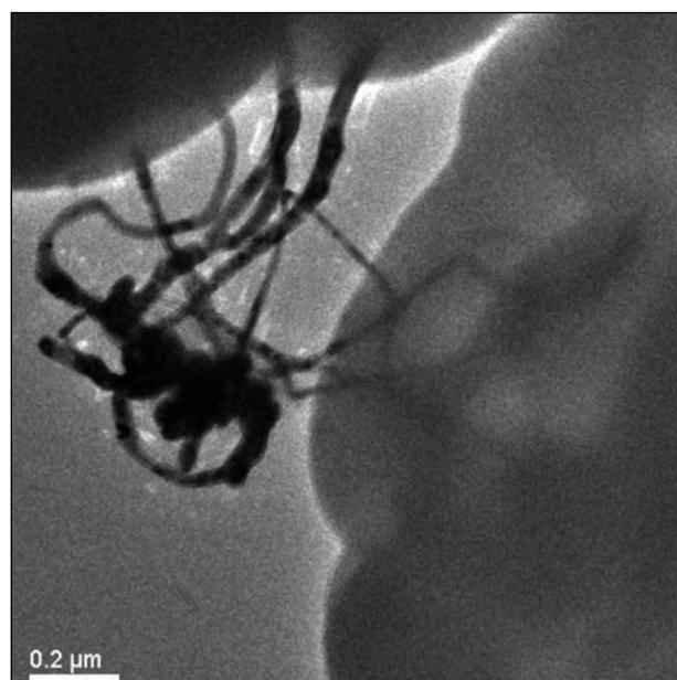
**Figure 7:** TEM images of particles gained by spray drying of an  $\text{Ag}/\text{SiO}_2$  sol, product deposited in collecting container.
