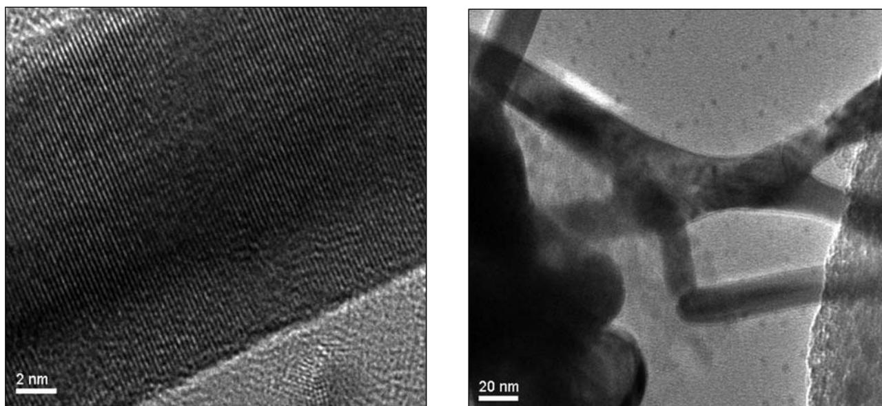
**Figure 8:** HRTEM images of particles gained by spray drying of an Ag/SiO<sub>2</sub> sol, product deposited in collecting container.
