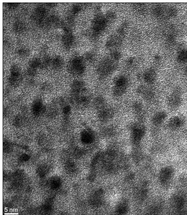
**Figure 2:** HRTEM image of a coating prepared from Ag/SiO<sub>2</sub> sol, as used for spray drying.
