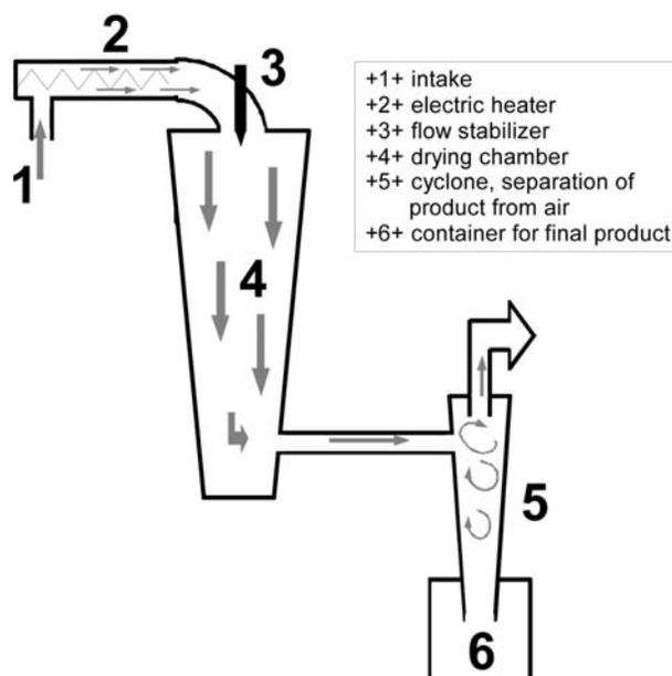
**Scheme 1:** Schematical drawing of the used spray dryer.
