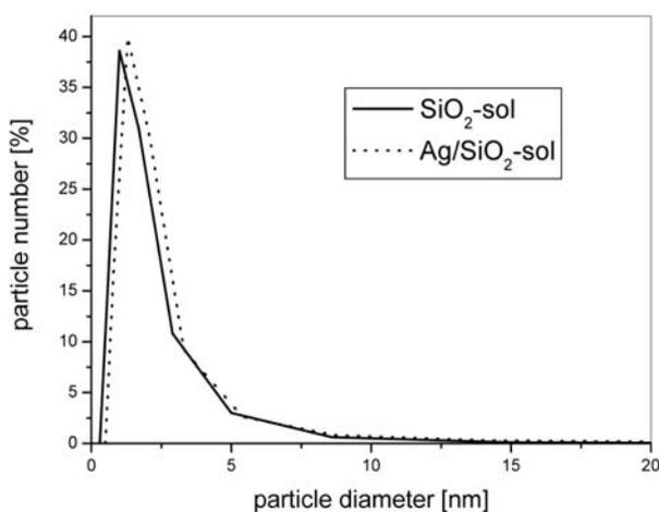
**Figure 1:** Particle size distribution of SiO<sub>2</sub> sols and SiO<sub>2</sub> in silver containing Ag/SiO<sub>2</sub> sols as used for spray drying.
