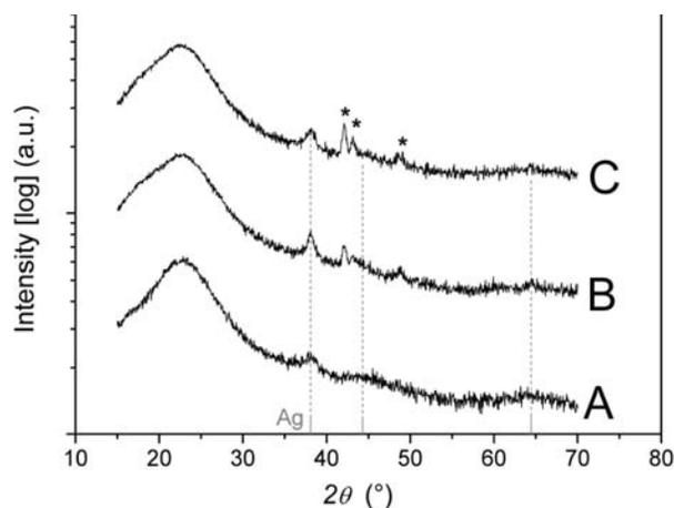
**Figure 6:** XRD patterns from the liquid sol (pattern A) and of dried powder samples gained from spray drying (pattern B for sample from collecting container and pattern C for sample from the cyclone). Reflections marked with an asterisk (\*) belong to the sample holder.
