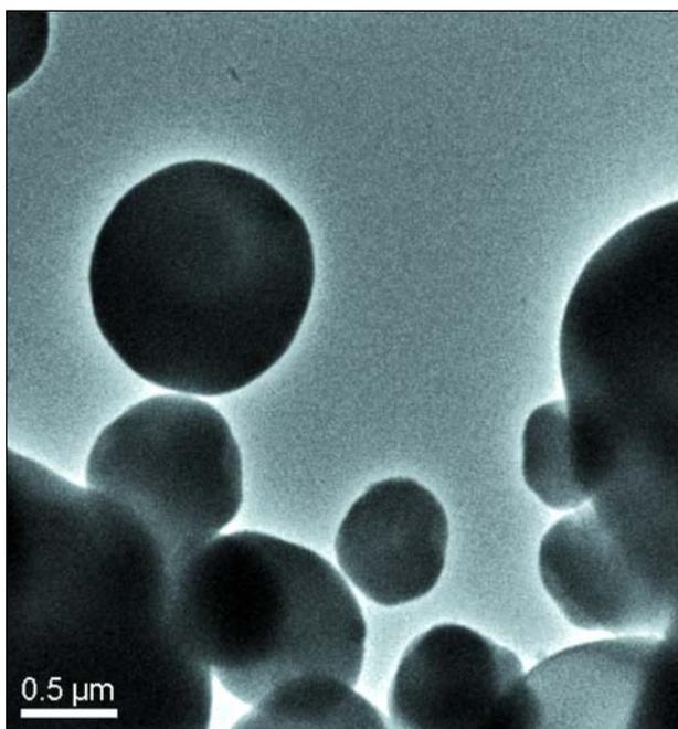
**Figure 3:** SEM image (above) and TEM image (below) of particles gained by spray drying of a SiO<sub>2</sub> sol.
