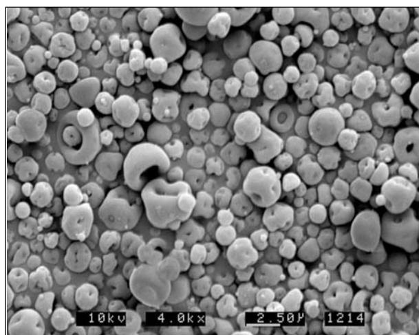
**Figure 4:** SEM image of particles gained by spray drying of an Ag/SiO<sub>2</sub> sol.
