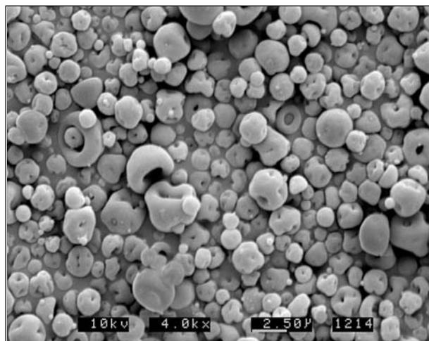
**Figure 4:** SEM image of particles gained by spray drying of an Ag/SiO<sub>2</sub> sol.
