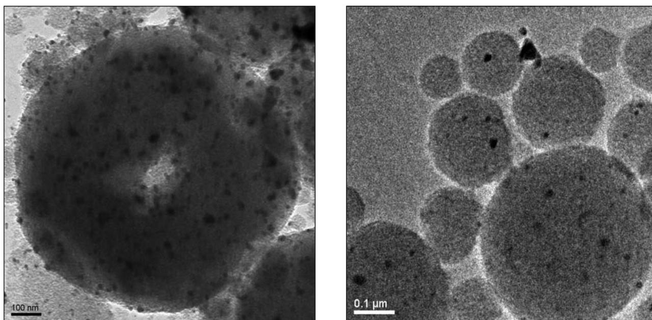
**Figure 9:** TEM images of particles gained by spray drying of an Ag/SiO<sub>2</sub> sol, product deposited in drying chamber.
