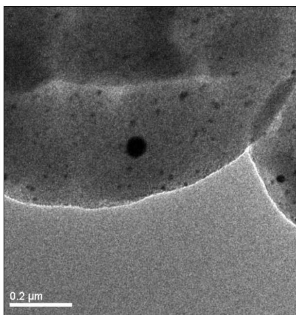
**Figure 5:** TEM image of particles gained by spray drying of an Ag/SiO<sub>2</sub> sol, product deposited in the collecting container.
