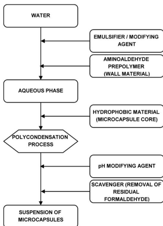
**Figure 1:** *In situ* polymerisation microencapsulation procedure in a 200 l reactor
