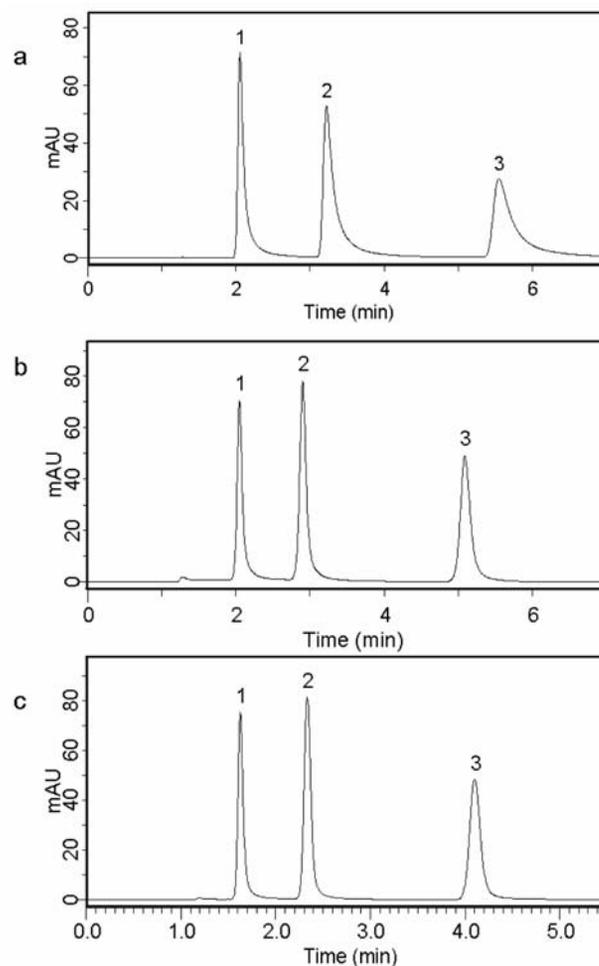
**Figure 8.** Chromatographic separation of catecholamines in 100% aqueous mobile phase conditions on (a) Symmetry C18 (b) ODS prepared and (c) polar-modified columns. Chromatographic conditions: mobile phase, 20 mM phosphate buffer, pH 7.0; flow rate, 1 mL · min<sup>-1</sup>; detection, UV 270 nm. Peaks: 1 – norepinephrine, 2 – epinephrine, 3 – dopamine.
