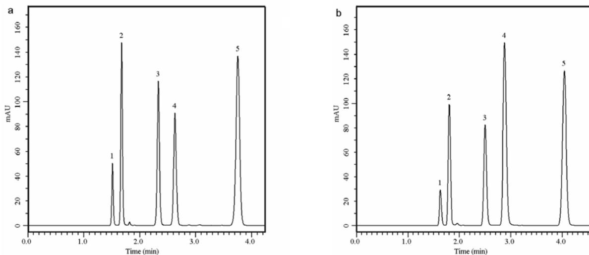
**Figure 5.** Silanophilic acidic probes on (a) ODS prepared and (b) polar-modified columns. Chromatographic conditions: mobile phase, MeCN:H<sub>2</sub>O, 1:1, plus 0.1% formic acid; flow rate, 1 mL · min<sup>-1</sup>; detection, UV 254 nm. Peaks: 1 – uracil, 2 – caffeine, 3 – sorbic acid, 4 – salicylic acid, 5 – propylparaben.
