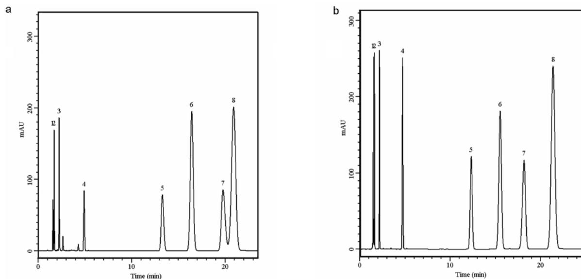
**Figure 3.** Chromatographic separation of neutral analytes using (a) ODS prepared and (b) polar-modified columns. Chromatographic conditions: mobile phase, MeCN:H<sub>2</sub>O, 60:40; flow rate, 1 mL · min<sup>-1</sup>; detection, UV 254 nm. Peaks: 1 – uracil, 2 – caffeine, 3 – phenol, 4 – toluene, 5 – butylbenzene, 6 – *o*-terphenyl, 7 – amylbenzene, 8 – triphenylene.
