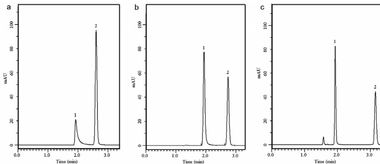
**Figure 4.** Chromatograms of pyridine and phenol on (a) Symmetry C18 (b) ODS prepared (c) polar-modified columns. Chromatographic conditions: mobile phase, acetonitrile:water, 1:1; flow rate, 1 mL · min<sup>-1</sup>; detection, UV 254 nm. Peaks: 1 – pyridine, 2 – phenol.
