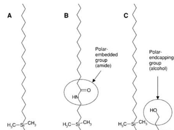
**Figure 1.** Representative structures for (A) a conventional ODS phase, (B) a polar-embedded phase, and (C) a polar-endcapped phase.
