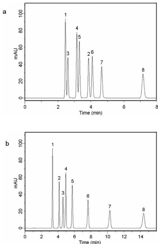
**Figure 9.** Separation of phenol derivatives on (a) ODS prepared and (b) polar-modified columns. Chromatographic conditions: mobile phase, 0.1% HCOOH in acetonitrile:0.1% HCOOH in H<sub>2</sub>O, 55:45; flow rate, 1 mL · min<sup>-1</sup>; detection, UV 280 nm. Peaks: **1** – phenol, **2** – 2-nitrophenol, **3** – 4-nitrophenol, **4** – 2-chlorophenol, **5** – 4-chlorophenol, **6** – 4-chloro-3-methylphenol, **7** – 2, 4-dichlorophenol, **8** – 2, 4, 6-trichlorophenol.
