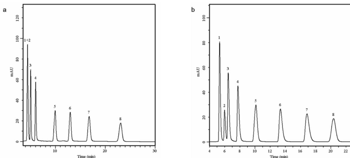
**Figure 6.** Separation of tricyclic antidepressants at pH 7.0 on (a) ODS prepared and (b) polar-modified columns. Chromatographic conditions: mobile phase, MeCN:MeOH:10 mM phosphate buffer, pH 7.0, 1:1:1; flow rate, 1 mL min<sup>-1</sup>; detection, UV 254 nm. Peaks: 1 – desmethyldoxepin, 2 – protriptyline, 3 – desipramine, 4 – nortriptyline, 5 – doxepin, 6 – imipramine, 7 – amitriptyline, 8 – trimipramine.
