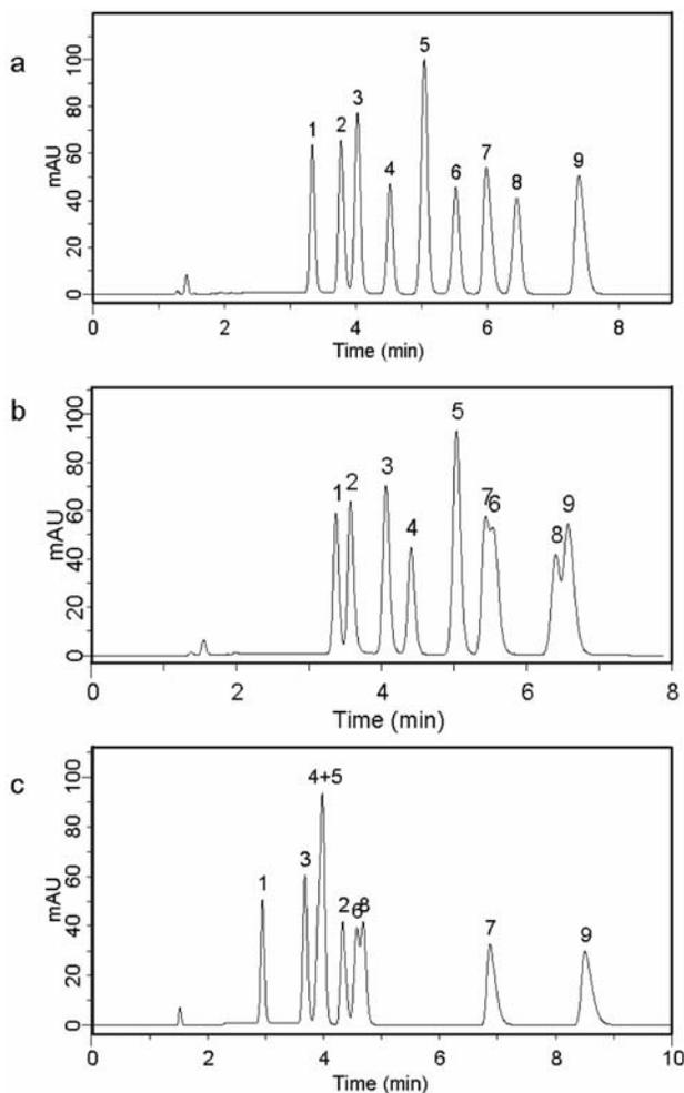
**Figure 7.** Chromatographic separation of tricyclic antidepressants and benzodiazepines on (a) ODS prepared (b) Luna C18 (2) and (c) XBridge C18 columns. Chromatographic conditions: mobile phase, 0.1% TFA in MeCN:0.1% TFA in H<sub>2</sub>O, 40:60; flow rate, 1 mL · min<sup>-1</sup>; detection, UV 254 nm. Peaks: 1 – nitrozepam, 2 – nordoxepin, 3 – alprazolam, 4 – diazepam, 5 – oxazepam, 6 – triazolam, 7 – nortriptyline, 8 – clonazepam, 9 – trimipramine.
