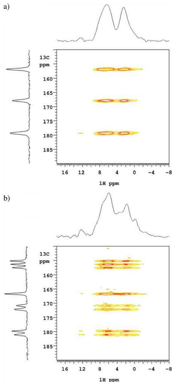
**Figure 4.** Two-dimensional  $^1\text{H}$ - $^{13}\text{C}$  HETCOR NMR spectra of indomethacin gamma (a) and alpha (b). Along the carbon-axis only the parts of the spectra containing carbonyl and carboxyl peaks are shown. Tiny cross-peaks at about 12 ppm along the proton-axis show that indeed protons of the carbonyl groups take part in the hydrogen bonds between the adjacent indomethacin molecules.
