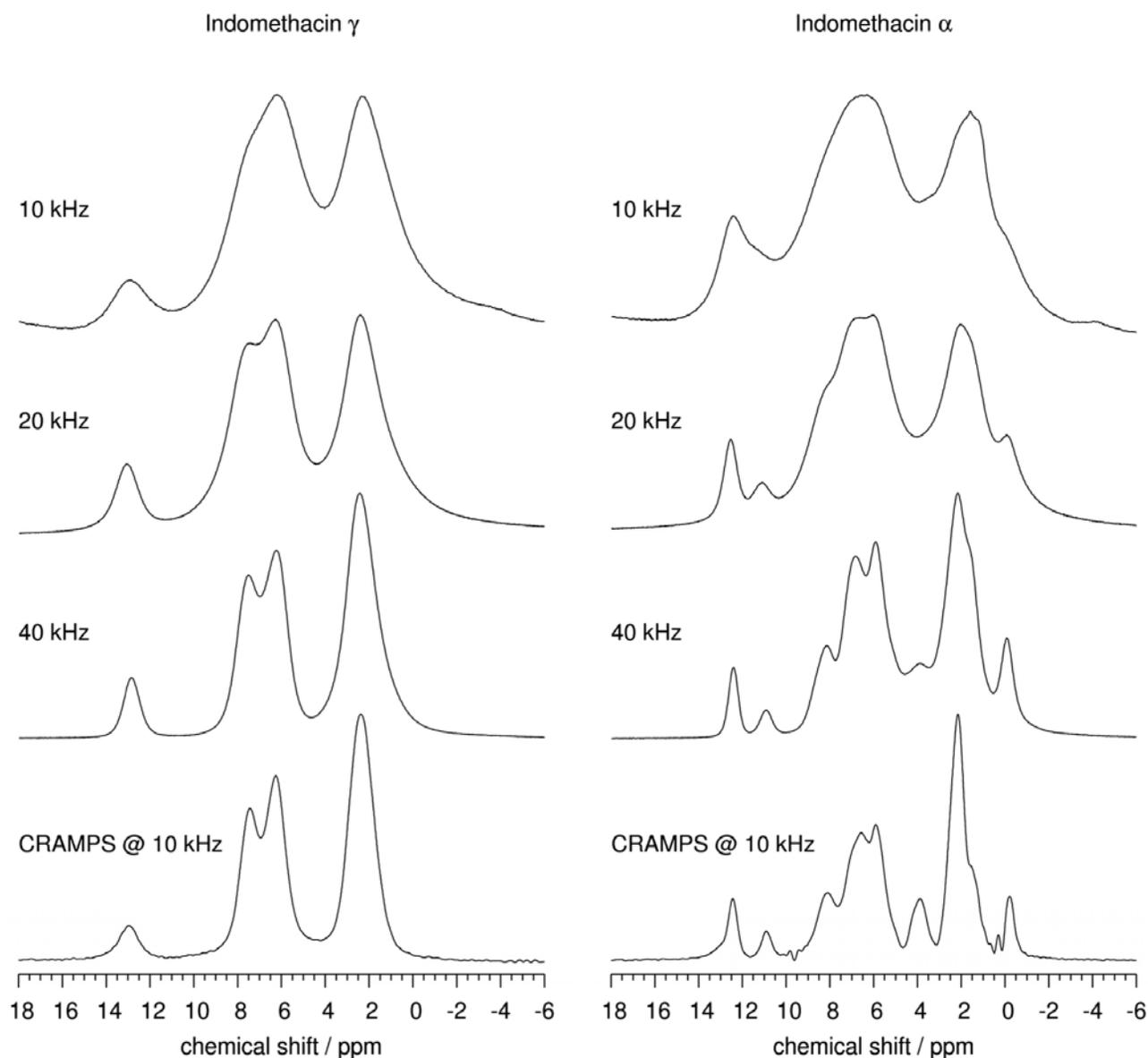
**Figure 3.**  $^1\text{H}$  MAS and CRAMPS NMR spectra of the two polymorphs of indomethacin. The sample rotation frequencies are indicated on the left of the spectra. The chemical shift axis for the CRAMPS spectra was scaled so that the peak positions within these spectra match the peak positions within the MAS spectra. Scaling factor was 2.08.
