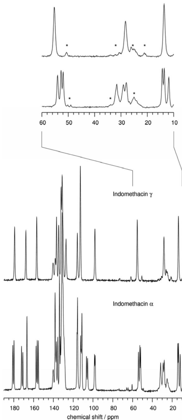
**Figure 2.**  $^1\text{H}$ - $^{13}\text{C}$  CPMAS NMR spectra of the two polymorphs of indomethacin. The inset enlarges the parts of the spectra, where one can clearly see that the numbers of molecules within the asymmetric units of form gamma and form alpha are different. Peaks or groups of peaks marked with asterisks are spinning-sidebands.
