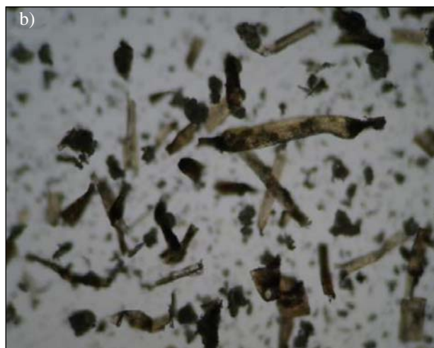
Figure 5: Effect of the drying temperature on the shape of the algal biomass. (a) Thermal treatment at 100 °C and (b) treatment at 200 °C [amplification X100]
