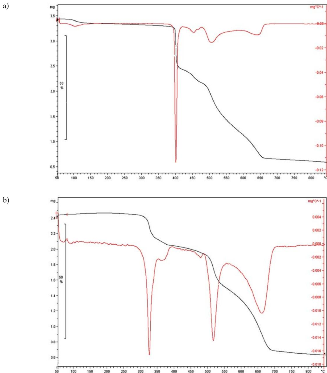
Fig. 6. Thermogravimetric (TG, black scale) and differential thermal analysis (DTA, red scale) of complex **1** (a) and complex **2** (b)
