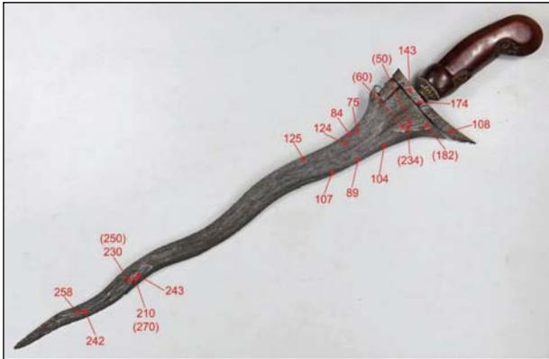
**Figure 2:** Photograph of kris N 32591, with locations and corresponding results of hardness measurements.
