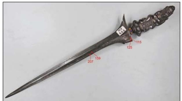
**Figure 4:** Photograph of kris MG 662, with locations and corresponding results of hardness measurements.
