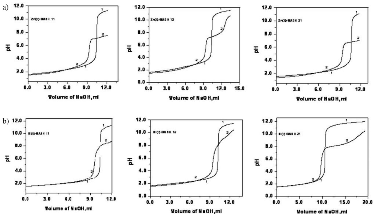
**Figure 3.** Simulated and experimental titration curves for (a) Zn(II)-SADH and (b) Ni(II)-SADH systems for 1:1, 1:2 and 2:1 compositions. (1.Simulated titration curve 2. Experimental titration curve)
