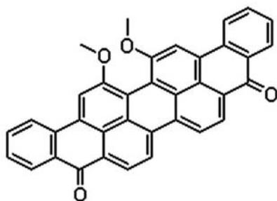
Fig. 1. Structural formula of Vat green 1 ( $C_{36}H_{20}O_4$ , C. I. 59825)
