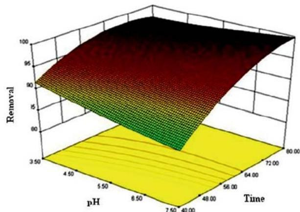
Fig. 4. Combined effect of time and pH on removal of the Vat green 1 dye.
