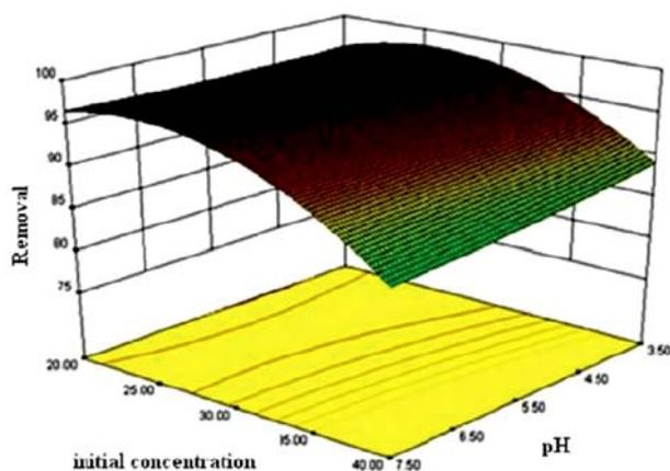
Fig. 5. Combined effect of pH and initial concentration on removal of the Vat green 1 dye.
