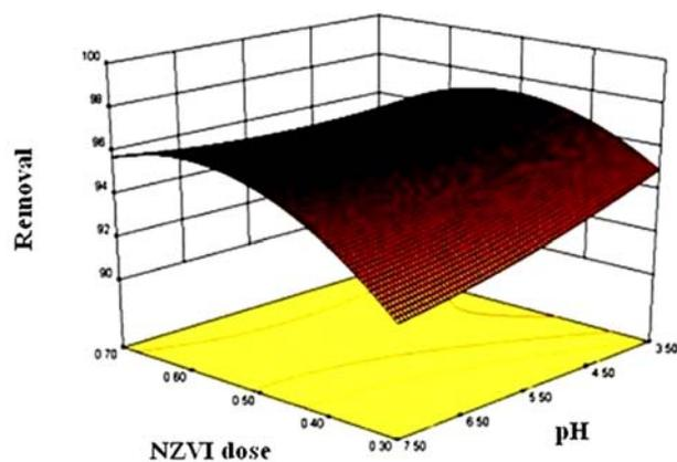
Fig. 3. Combined effect of NZVI dose and pH on removal of the Vat green 1 dye.
