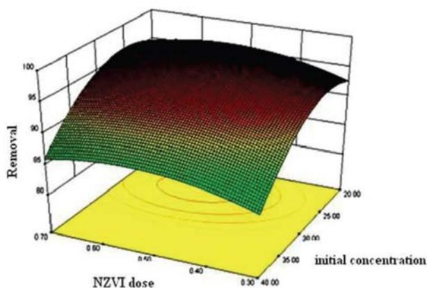
Fig. 7. Combined effect of NZVI dose and initial concentration on removal of the Vat green 1 dye.
