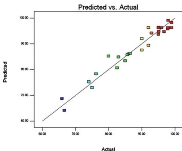
Fig 2. Actual and predicted values of removal of Vat green 1 by NZVI ( $R^2 = 0.95$ ).
