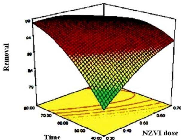
Fig. 6. Combined effect of NZVI dose and time on removal of the Vat green 1 dye.
