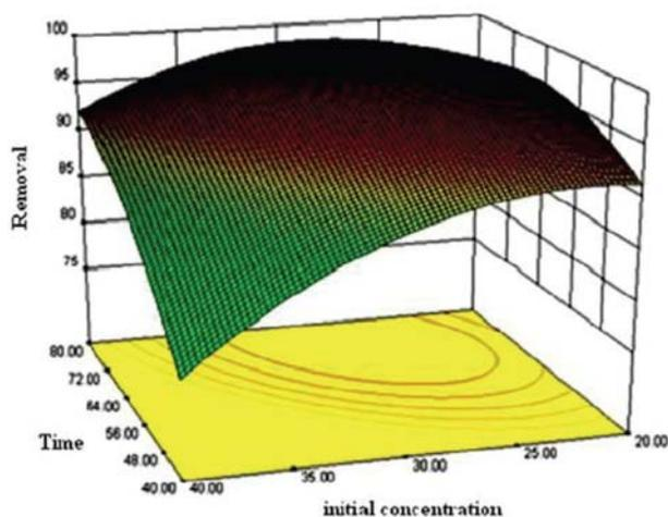
Fig. 8. Combined effect time and initial concentration on removal of the Vat green 1 dye.
