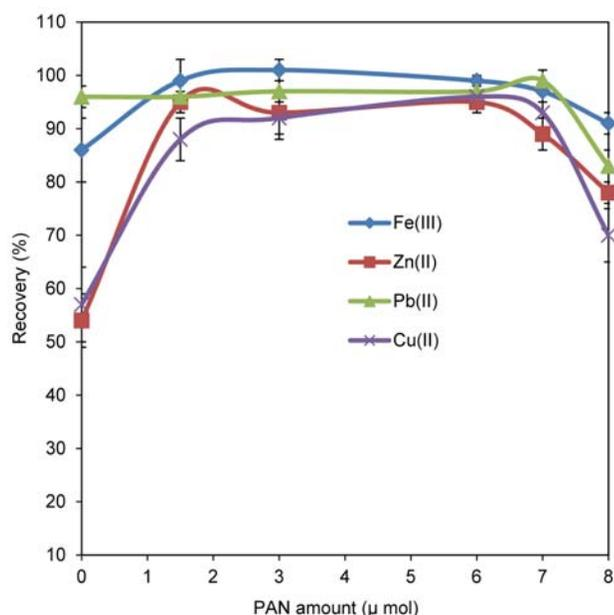
**Figure 2.** Effect of PAN amount on the recovery of studied metal ions (volume = 100 mL, n = 4).
