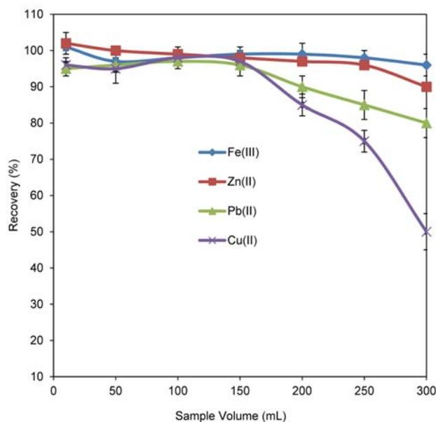
**Figure 3.** Effect of sample volume on the recovery of studied metal ions (n = 4).
