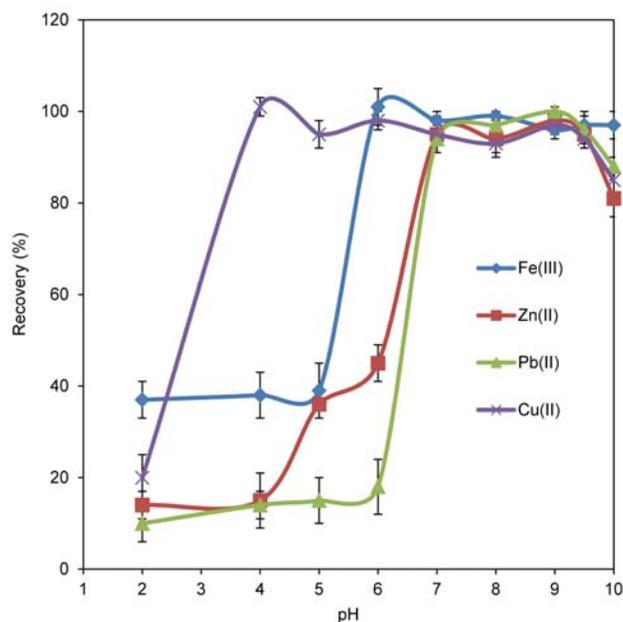
Figure 1. Effect of pH on the recovery of studied metal ions (volume = 100 mL, n = 4)
