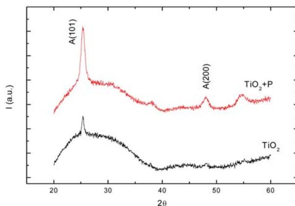
Figure 2: XRD pattern of TiO<sub>2</sub> thin films (A:anatase).
