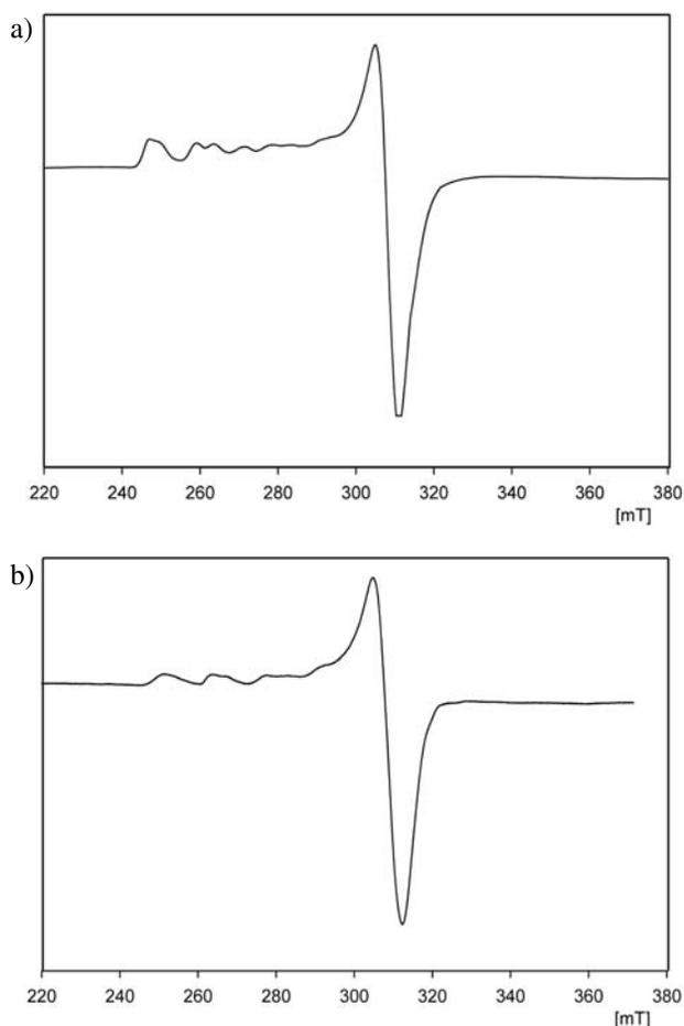
**Figure 3.** EPR spectra of Cu(II)/nicotine system (ratio 1:1) at pH = 3.5 (**3a**) and 6.0 (**3b**) (apart of signal of the complex the Cu<sup>2+</sup> signal exists).
