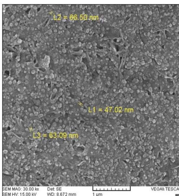
Figure 5. SEM micrograph of nano- $\gamma$ -ASA catalyst.
