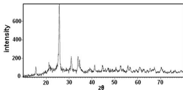
Figure 2. XRD pattern of nano- $\gamma$ -ASA catalyst.
