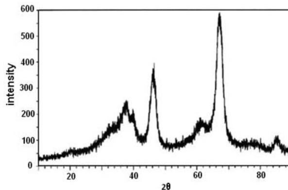
**Figure 1.** XRD pattern of nano- $\gamma$ -alumina catalyst.
