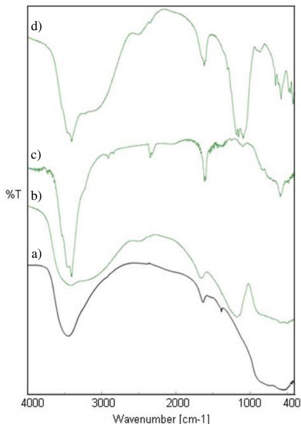
Figure 3. FT-IR spectra of a) alumina b) ASA c) nano- $\gamma$ -alumina d) nano- $\gamma$ -ASA catalysts.
