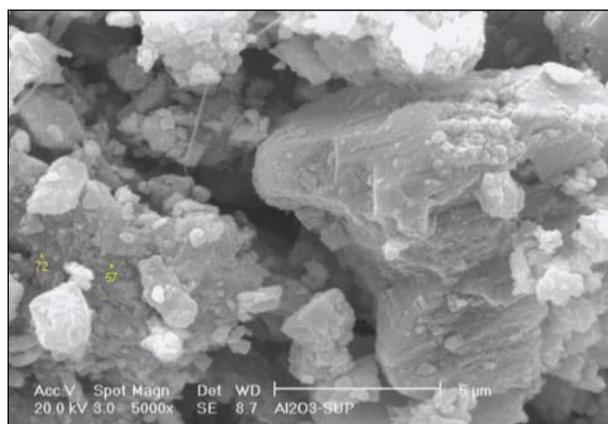
Figure 4. SEM micrograph of nano- $\gamma$ -alumina catalyst.
