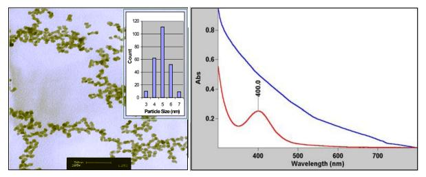
Figure 5. TEM, Particle Size and UV-vis Analysis of Pd- Nanoparticles (Reprinted with the permission from ref. 11, copyright, 2005, American Chemical Society).
