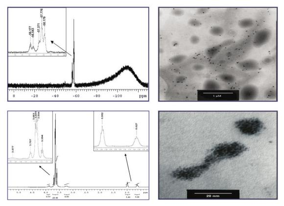
Figure 3. <sup>29</sup>Si-NMR and TEM images of PEG-substituted siloxane 2 (Reprinted with the permission from ref. 11, copyright, 2005, American Chemical Society).
