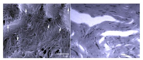
Figure 2. TEM image of the centrifuged reaction mixture silver nanoparticles incubated with collagen type 1.
