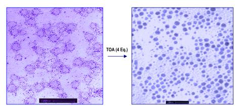
Figure 1. TEM image of the centrifuged reaction mixture of resulting silver nanonecklaces and and their conversion to nanocrystals (Reprinted with the permission from ref. 10, copyright, 2004, American Chemical Society).
