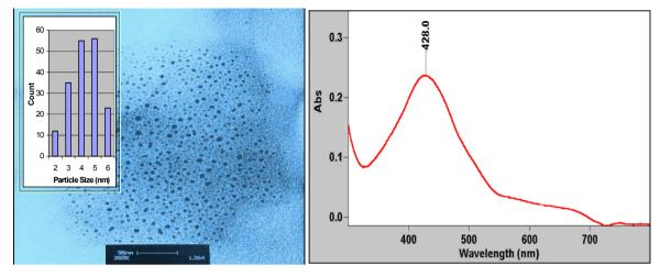
Figure 4. TEM, Particle Size and UV-vis Analysis of Ag Nanoparticles (Reprinted with the permission from ref. 11, copyright, 2005, American Chemical Society).
